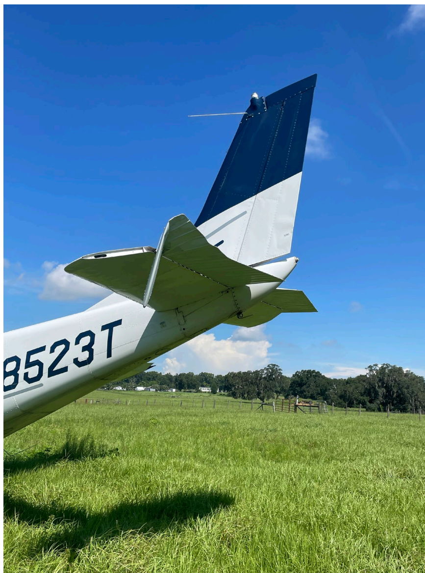
Photograph 2 - View of left elevator showing damage (Courtesy of FAA)
