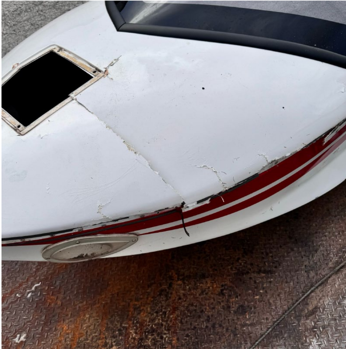
Photograph 3 - Impact damage - cracked forward hull (Courtesy of FAA)
