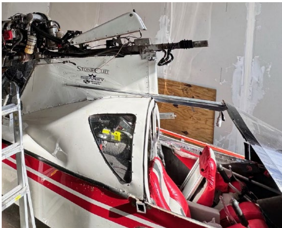
Photograph 2 - Impact damage - bent aircraft structure (Courtesy of FAA)
