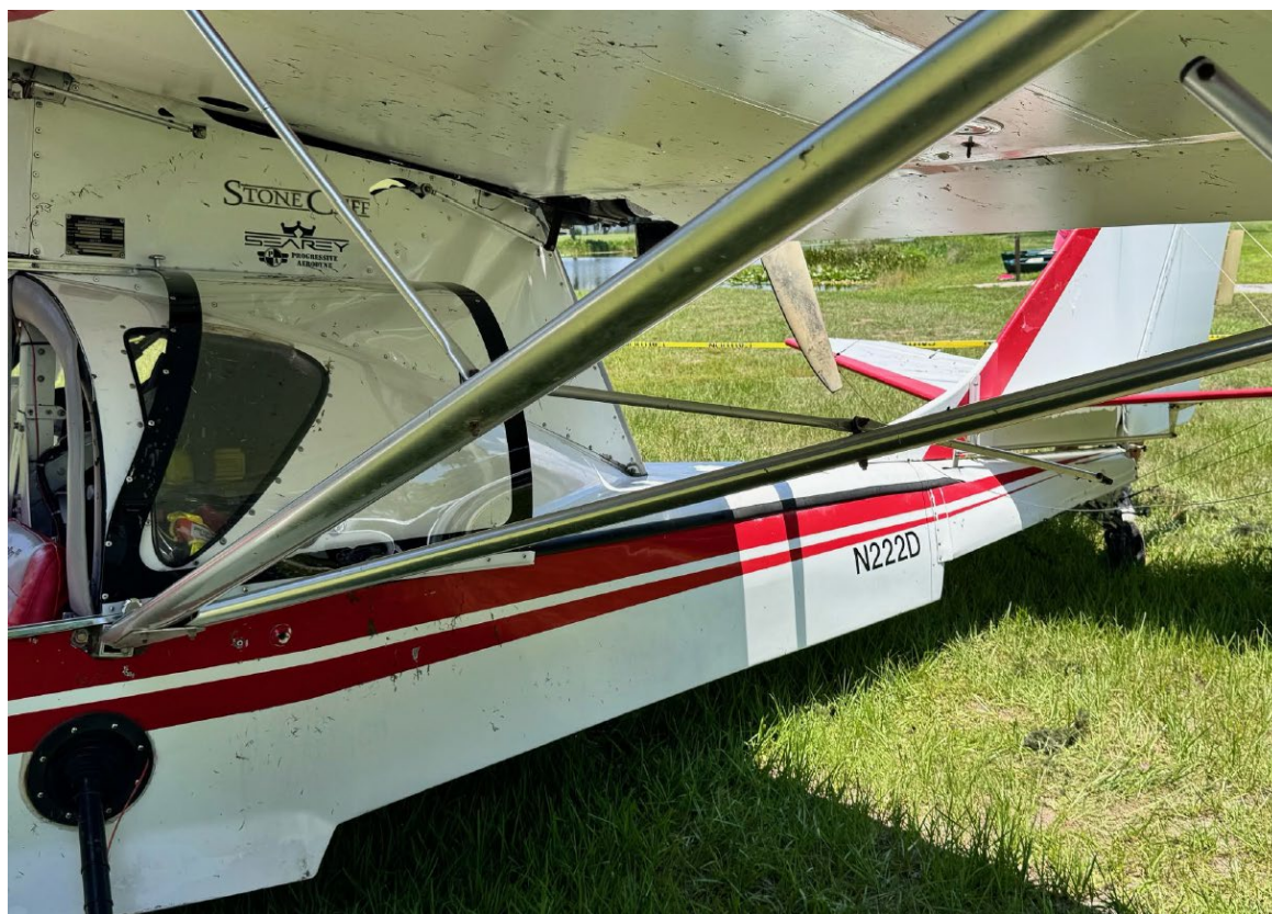
Photograph 4 - Impact damage - bent aircraft structure (Courtesy of FAA)
