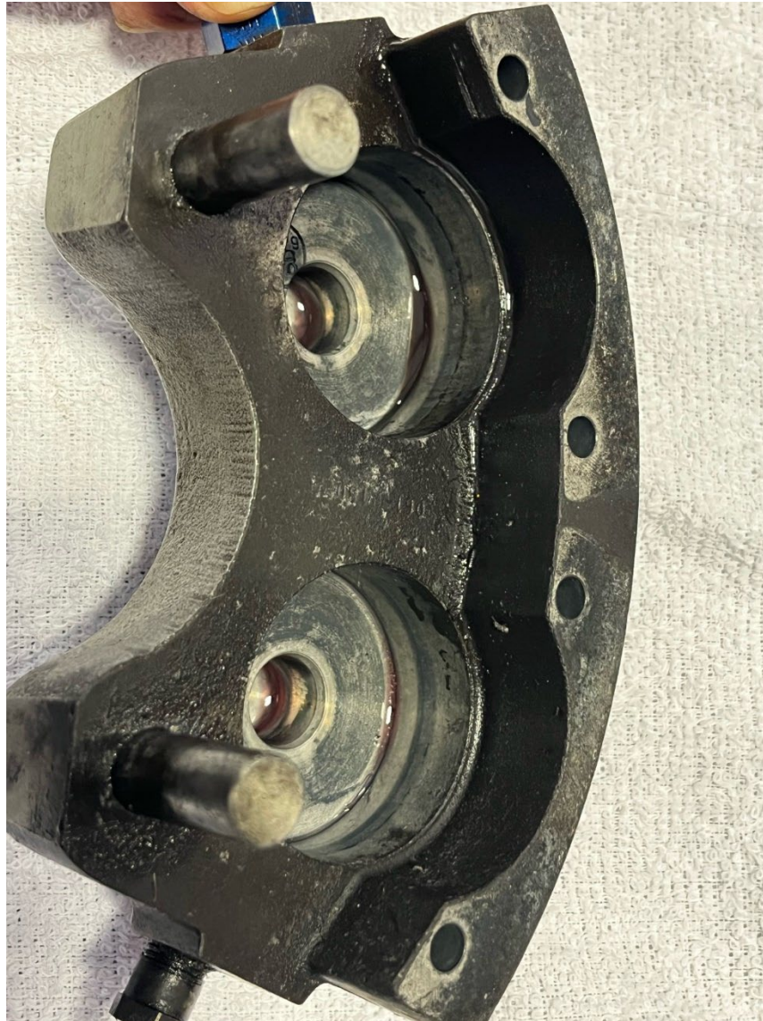
Photograph 8 - Disassembled right brake caliper (Courtesy of mechanic)
