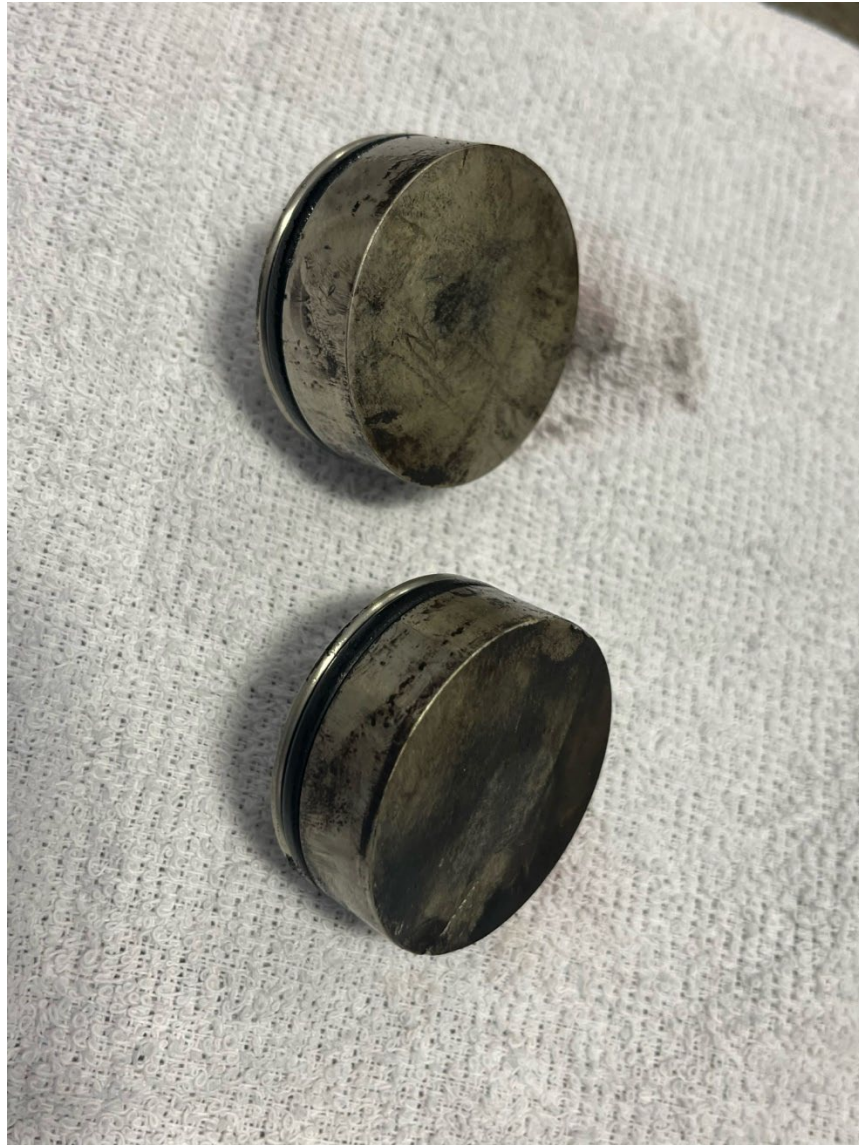
Photograph 9 - Right brake piston (Courtesy of mechanic)
