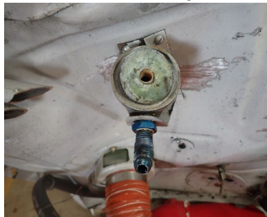
Photograph of gascolator screen.
