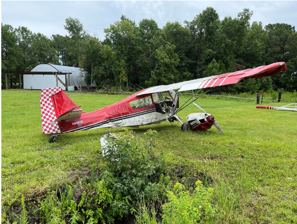
Photograph 2 - Deformation noted to fuselage (Courtesy of FAA)
