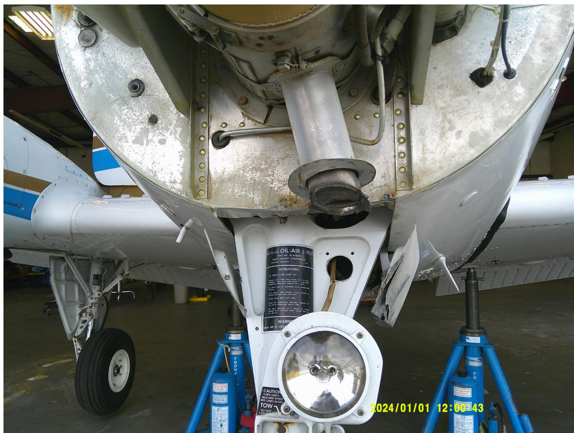
Photograph 1 - Damage to Bulkhead (Courtesy of FAA)
