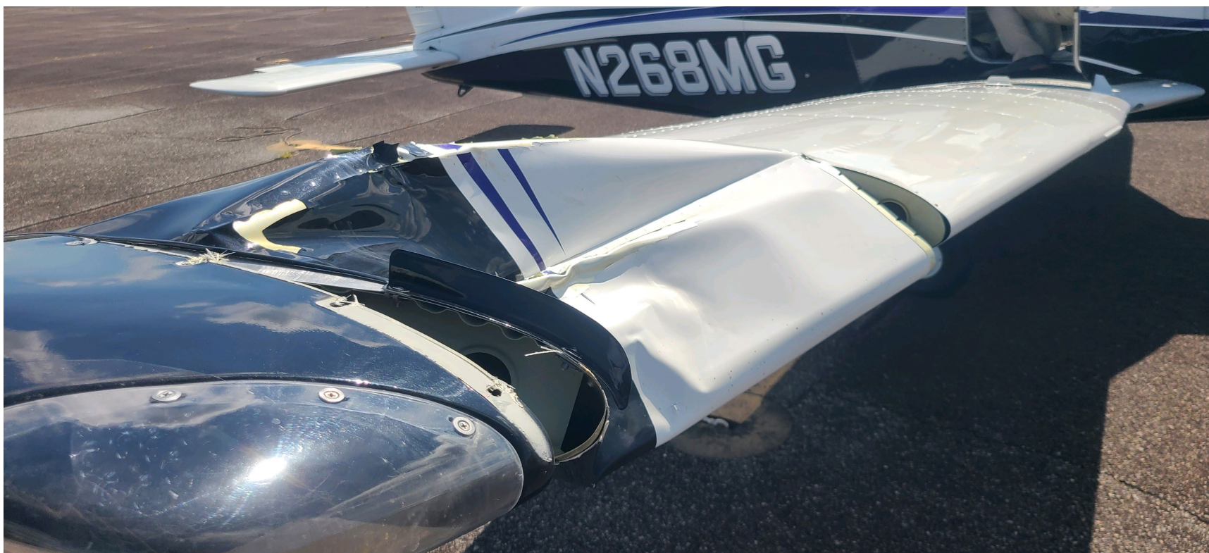
Photograph 2 – View of the damage to the right wing. (Courtesy of FAA)
