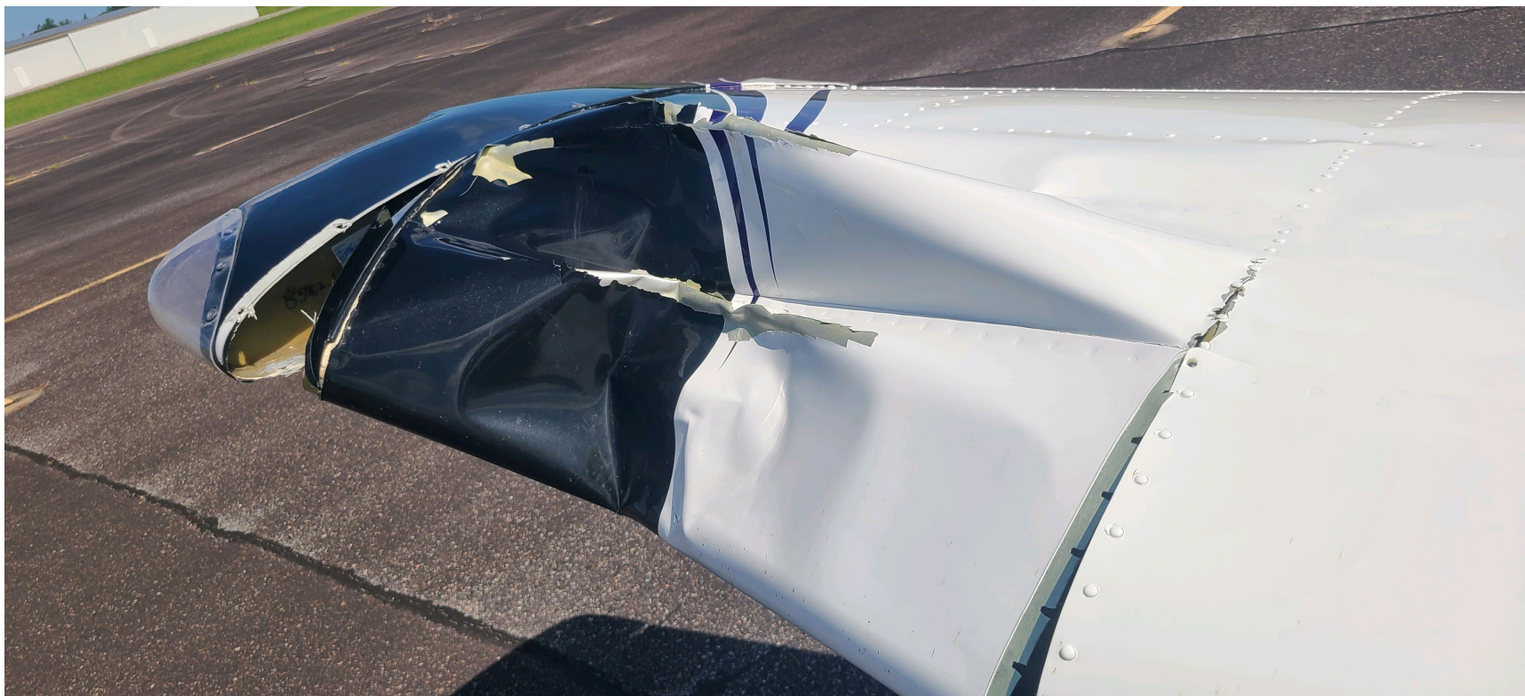
Photograph 3 – View of the damage to the right wing. (Courtesy of FAA)
