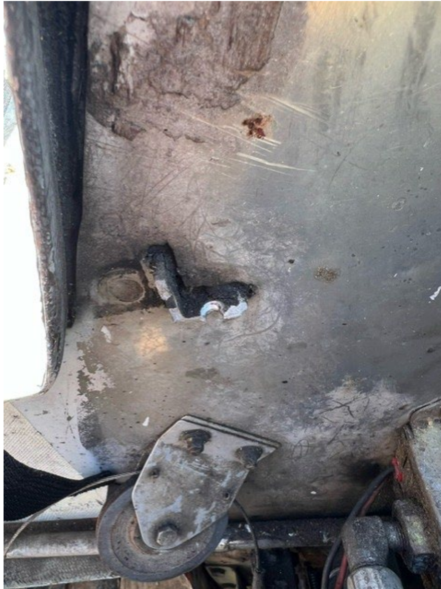
Photograph 2 - Sheared Engine mount 1 (Courtesy of pilot)
