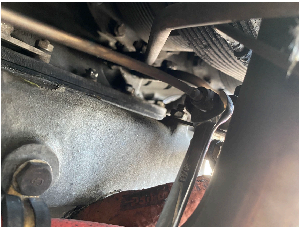
Photograph 2 - Loose Fuel Line B-Nut (FAA Photo)
