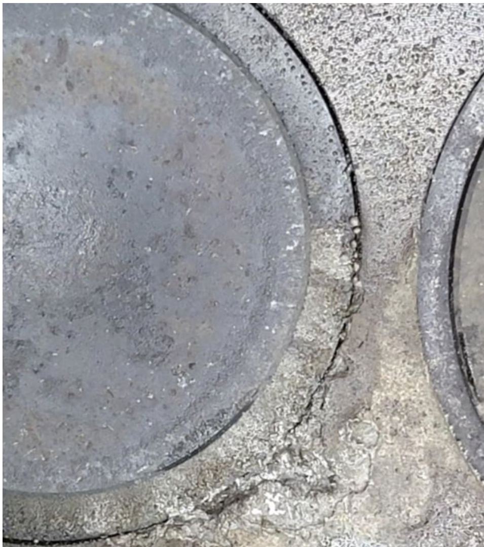
Photograph 2 - Damage to No. 3 cylinder. (Courtesy of FAA)
