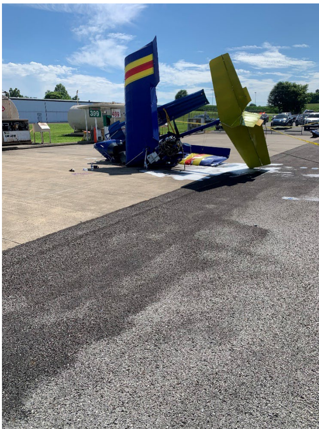
Photograph 2 - left side view of crashed airplane (Courtesy of FAA)
