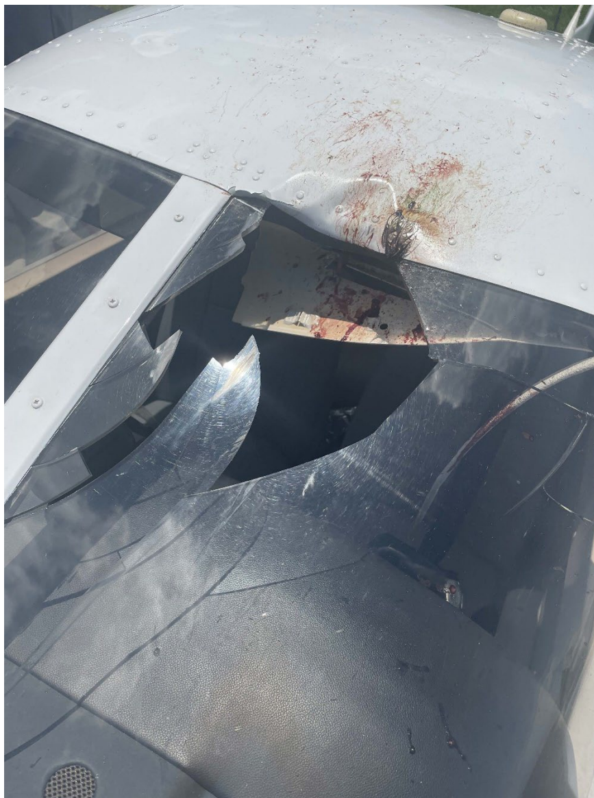
Photograph 2 - Postaccident view of bird impact (Courtesy of pilot)
