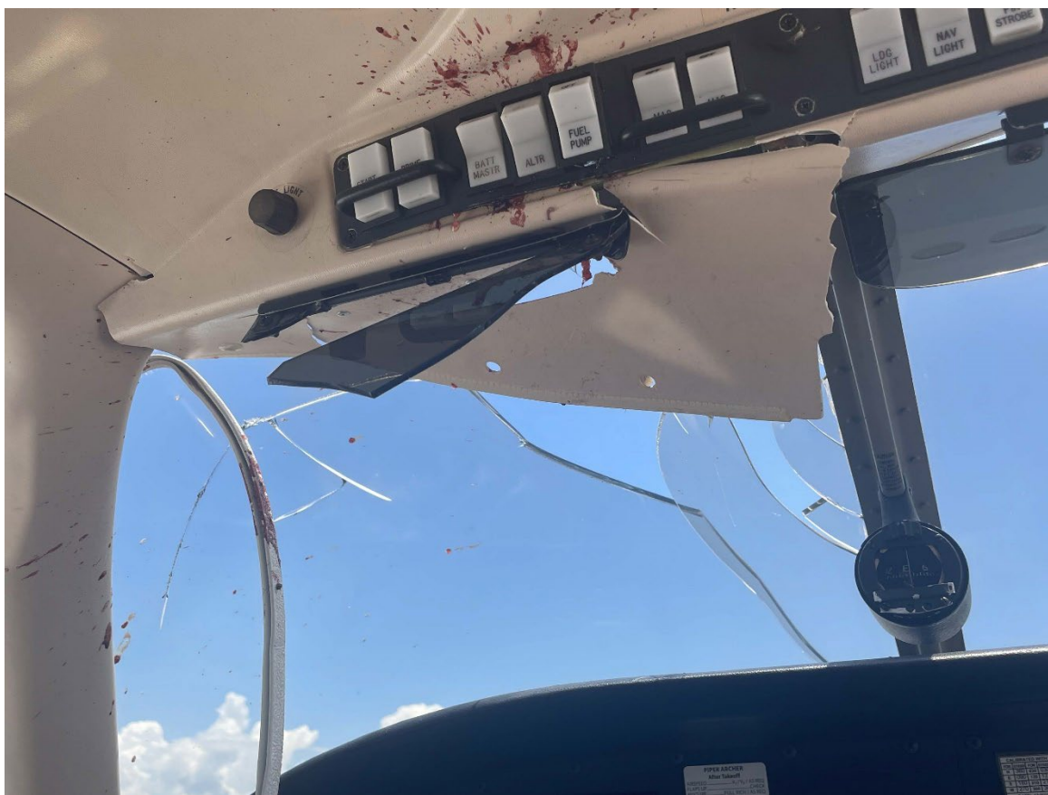
Photograph 3 - Bird impact damage from flight deck (Courtesy of pilot)
