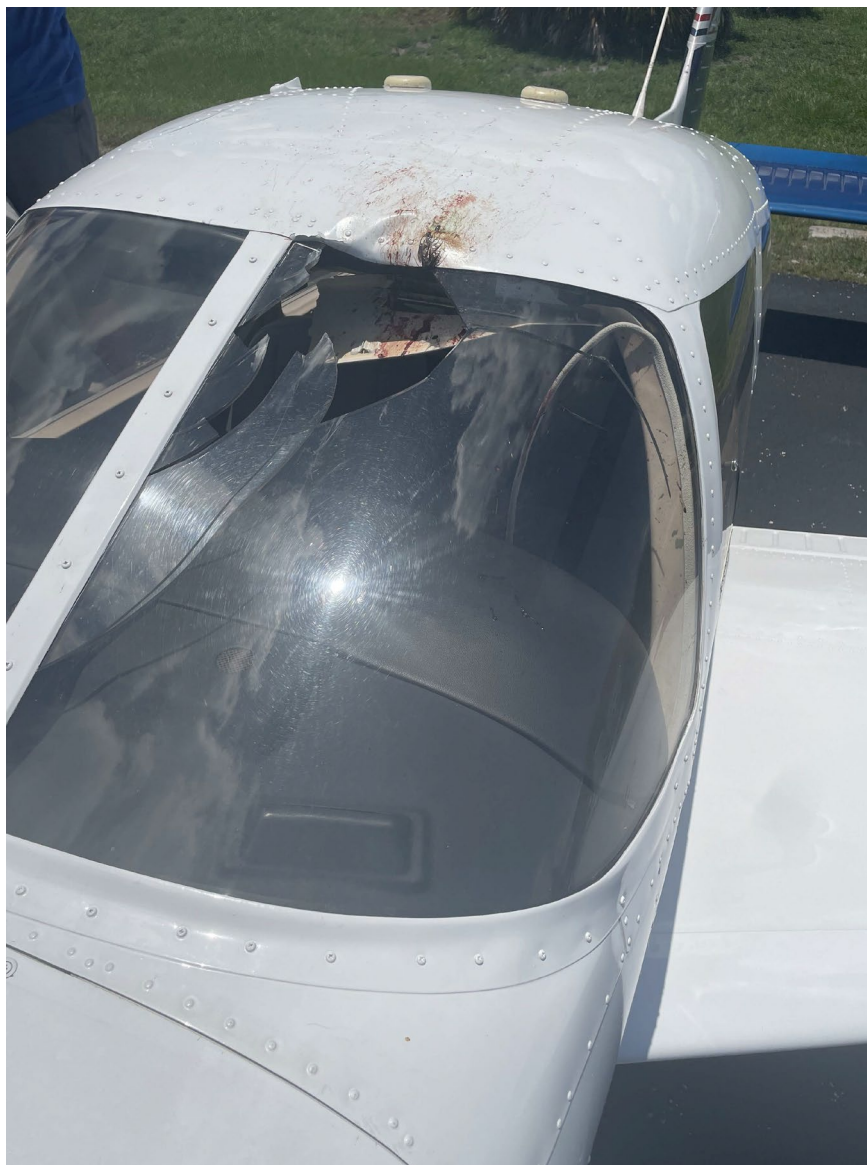
Photograph 1 - Postaccident view of bird impact (Courtesy of pilot)
