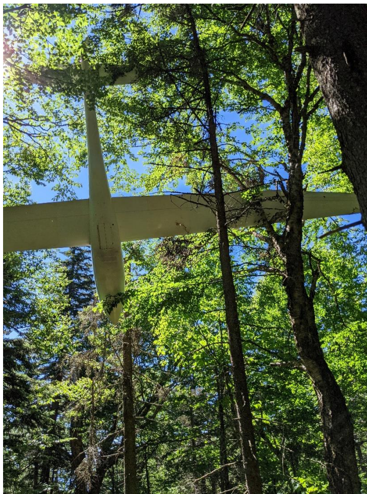
Photograph 2 - Glider in tree canopy with visible damage to right wing (Courtesy of FAA)
