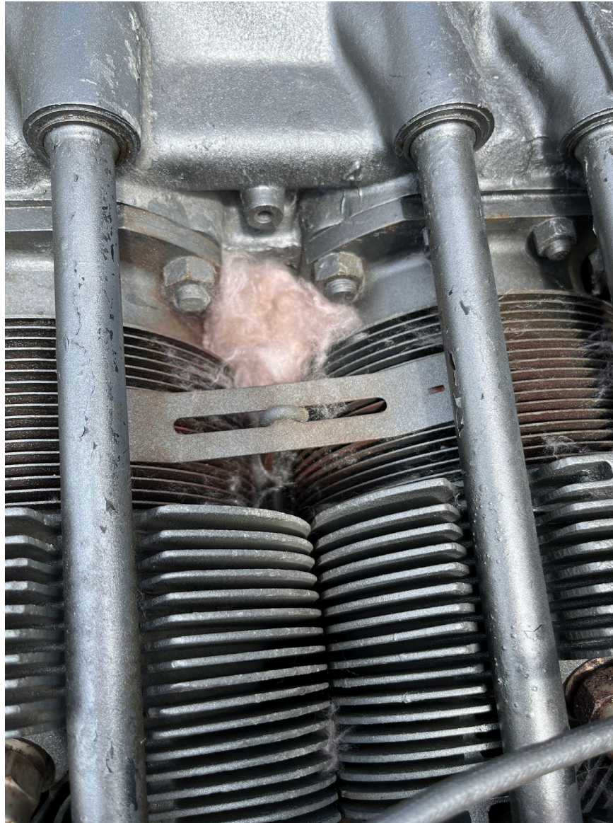
Photograph 4 - Residential-type insulation noted in engine area (Courtesy of FAA)
