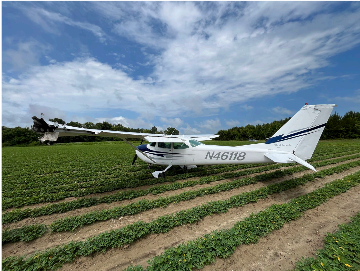
Photograph 1 - Left wing impact damage and aileron separation noted (Courtesy of FAA)
