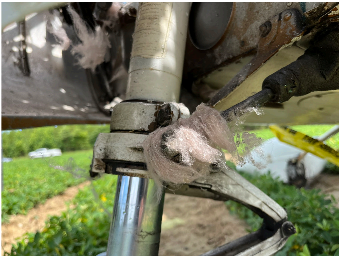
Photograph 3 - Residential-type insulation noted on nose landing gear (Courtesy of FAA)
