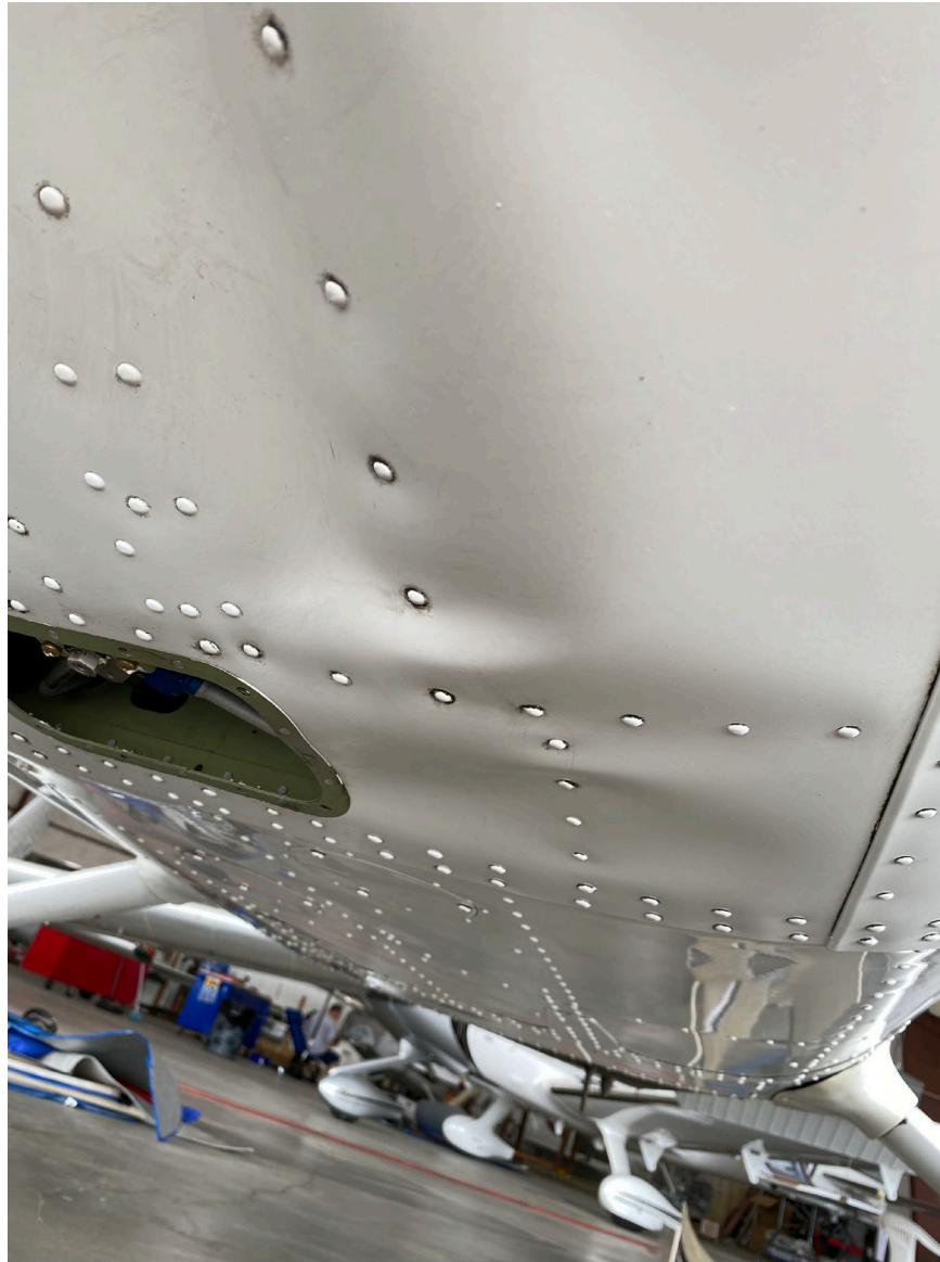
Photograph 2 - Postaccident lower fuselage damage (Courtesy of FAA)
