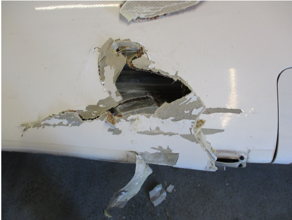
Photograph 2 - Closeup of leading edge wing damage. (Courtesy of Pilot/Owner)
