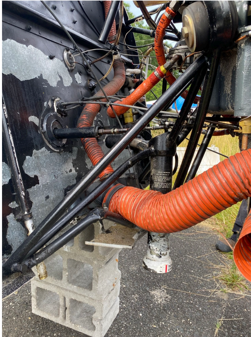
Photograph 2 - Deformation noted to engine mount (Courtesy of FAA)
