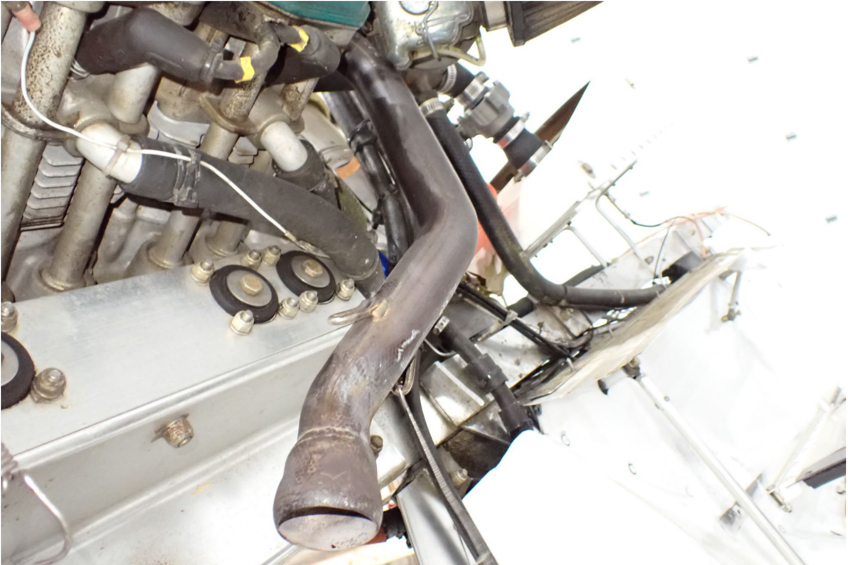
Photograph 14 - No. 4 exhaust riser
