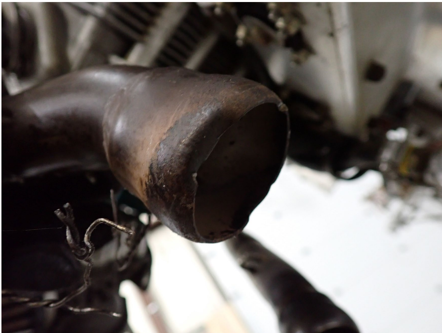
Photograph 7 - No. 1 exhaust riser end
