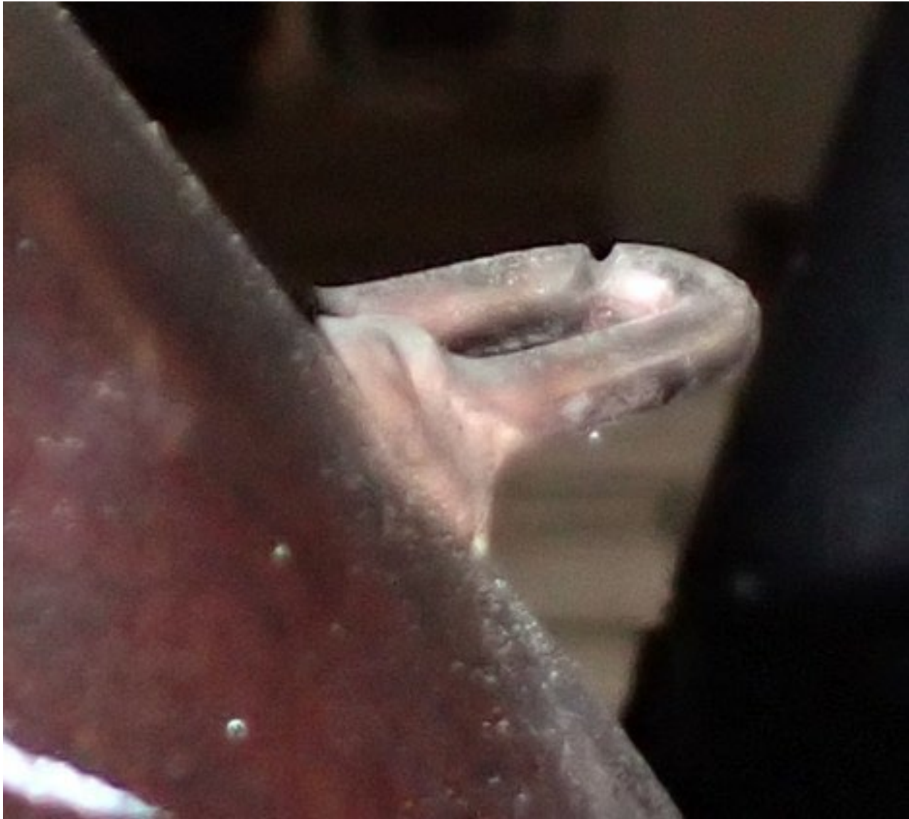
Photograph 10 - No. 3 exhaust riser spring attach loop
