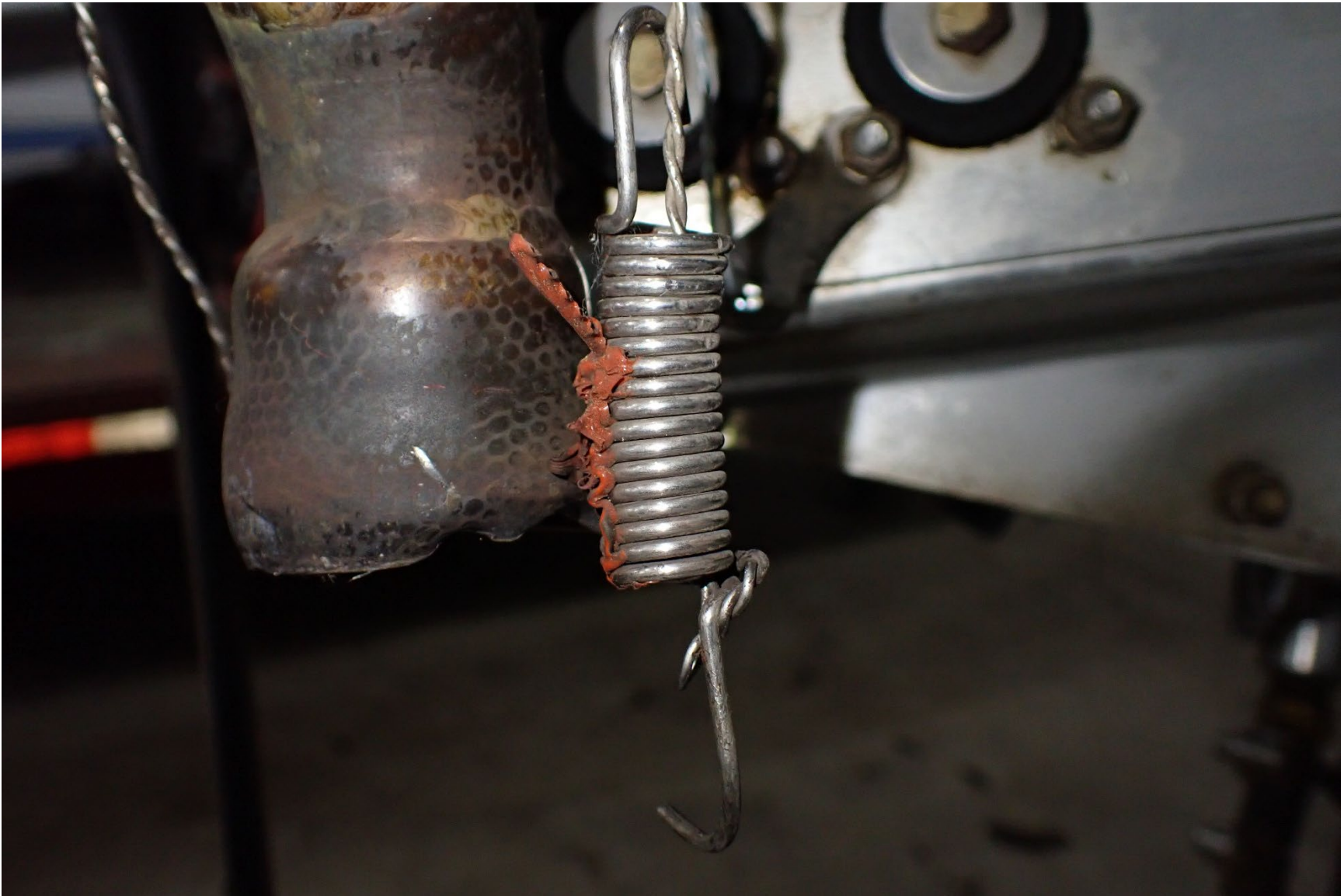
Photograph 13 - No. 2 exhaust spring
