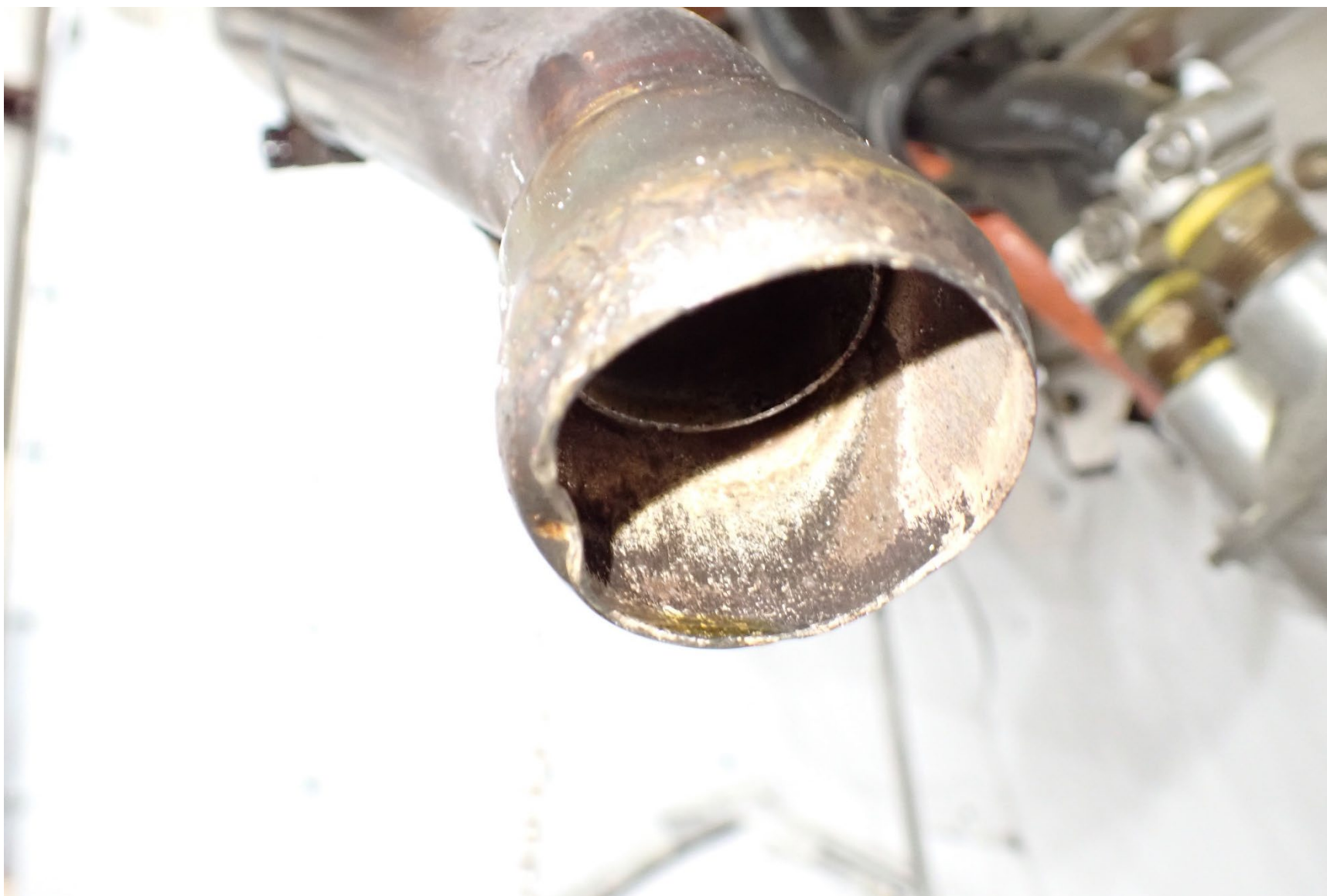
Photograph 9 - No. 3 exhaust riser end
