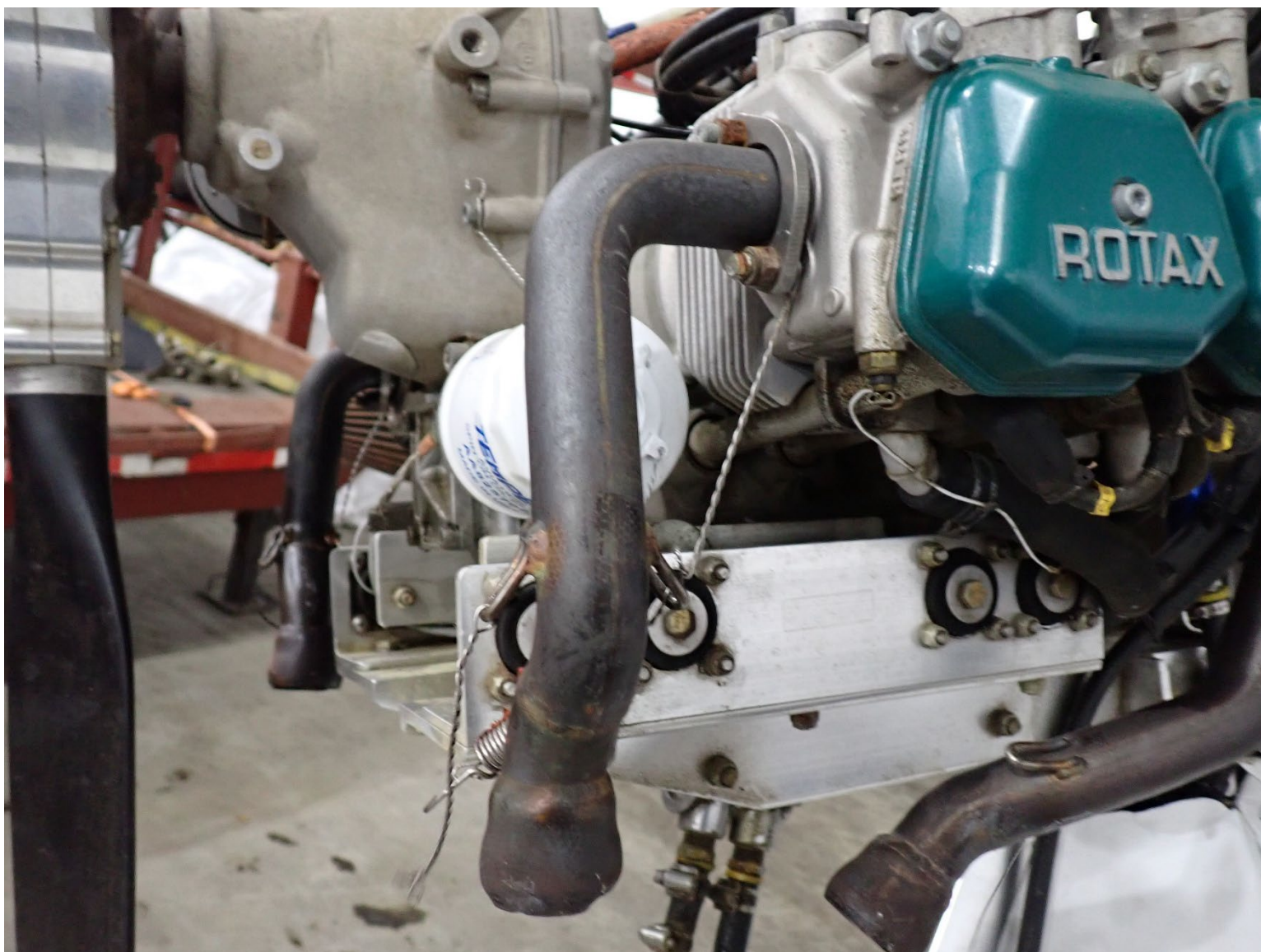
Photograph 11 - No. 2 exhaust riser
