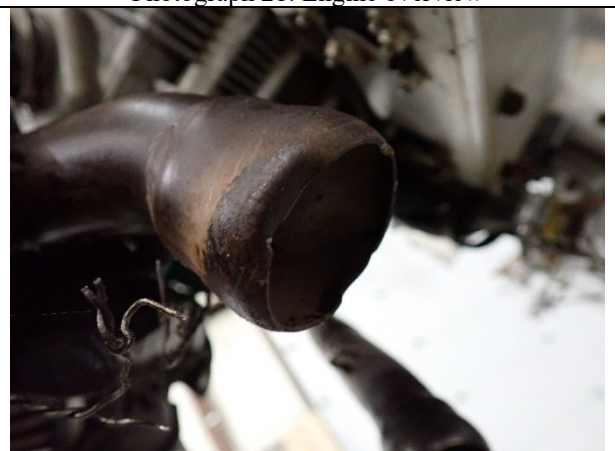
Photograph 23: No. 1 cylinder exhaust riser end
