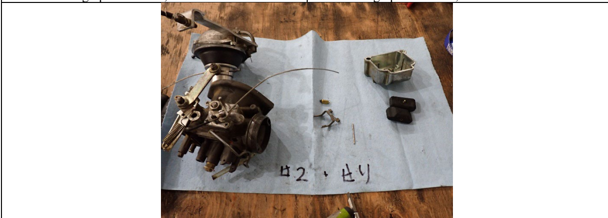
Photograph 19: No. 2, No. 4 carburetor after disassembly
