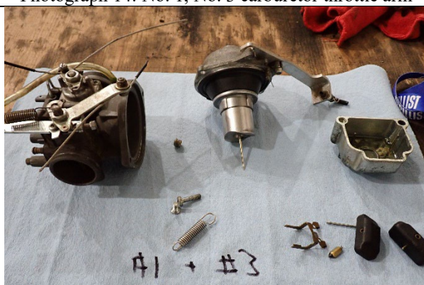
Photograph 16: No. 1, No. 3 carburetor after disassembly
