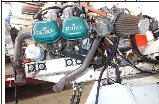
Photograph 30: No. 4 cylinder exhaust riser
