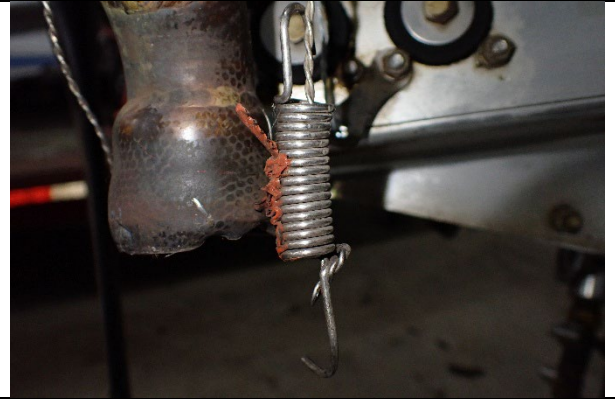
Photograph 27: No. 2 cylinder exhaust spring
