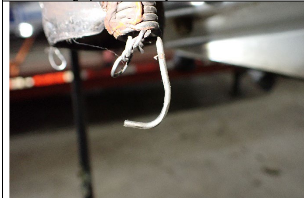
Photograph 28: No. 2 cylinder exhaust spring end
