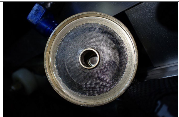
Photograph 4: Fuel strainer screen
