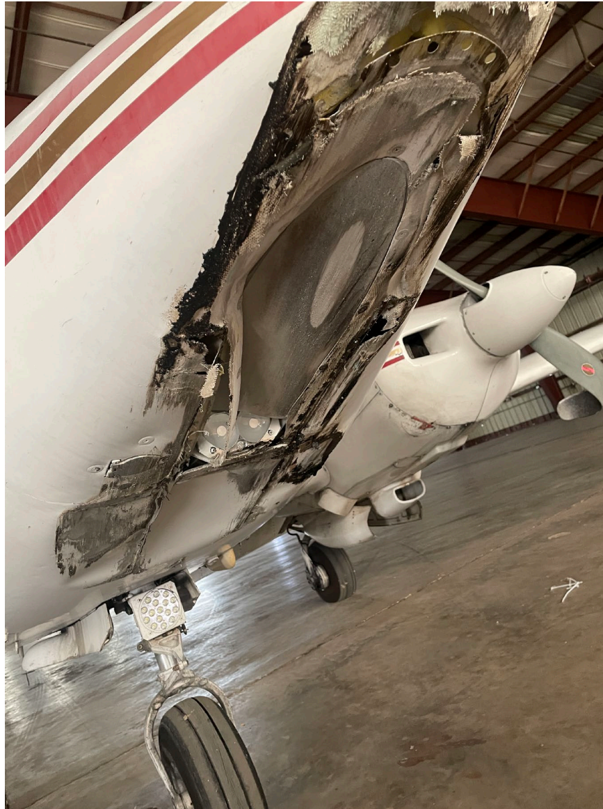
Photograph 3 - View of damage to the nose of the airplane. (Courtesy of FAA)
