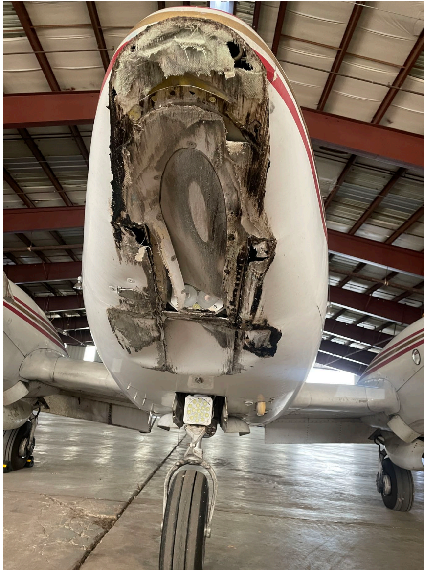
Photograph 2 - View of damage to the nose of the airplane. (Courtesy of FAA)
