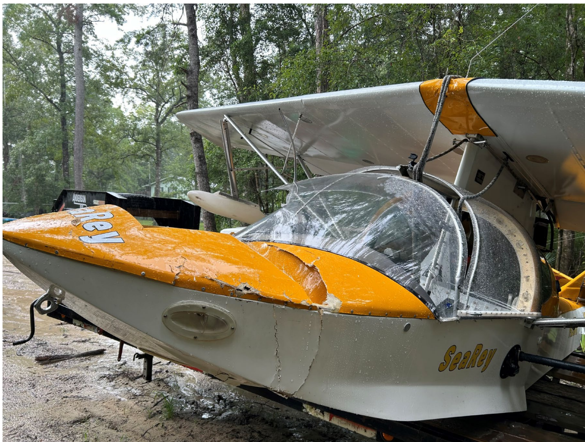
Photograph 2 - Hull Damage (Courtesy of Pilot)
