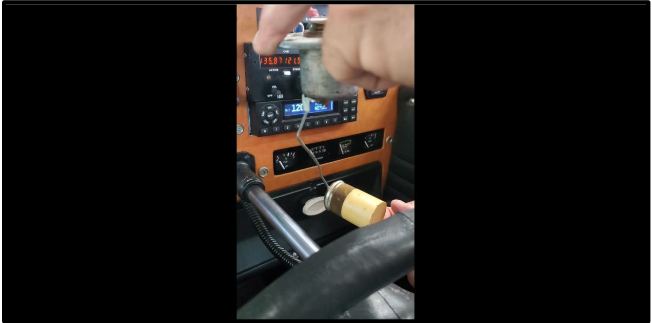
Figure 1: Electrical and Operational Testing of Fuel Quantity Indicating System. View Depicts Left Fuel Quantity Gauge Indicating Empty When fuel Sending Unit was Fully Extended
