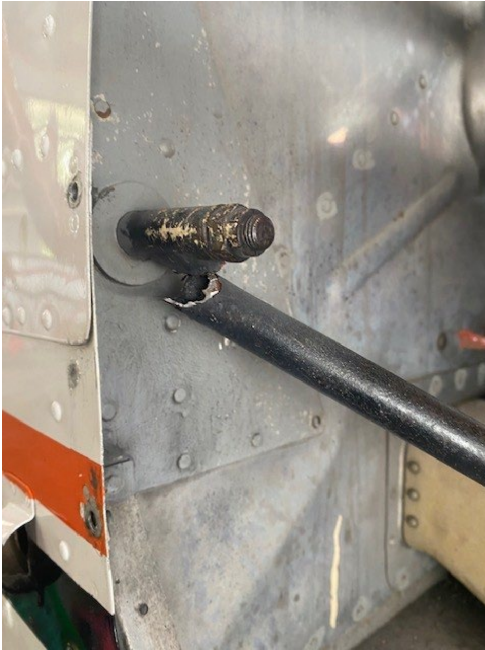
Figure 3: View Showing the Fractured Engine Mount Tube.
