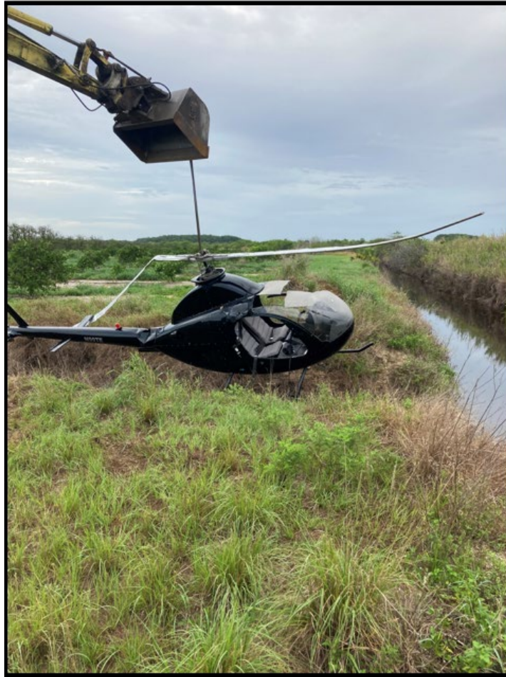
Figure 2: View of the Helicopter During Recovery. Note the Damage to the Tailboom.
