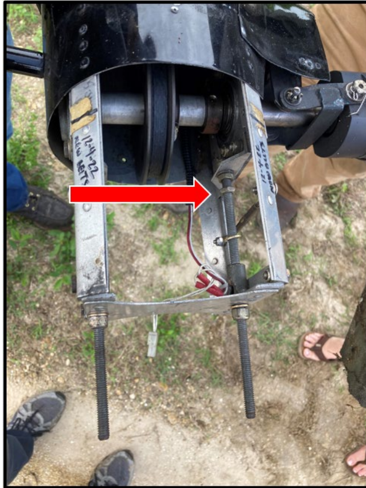
Figure 3: Arrow Points to Tail Rotor Drive Belt Jam Nut Out of Position.
