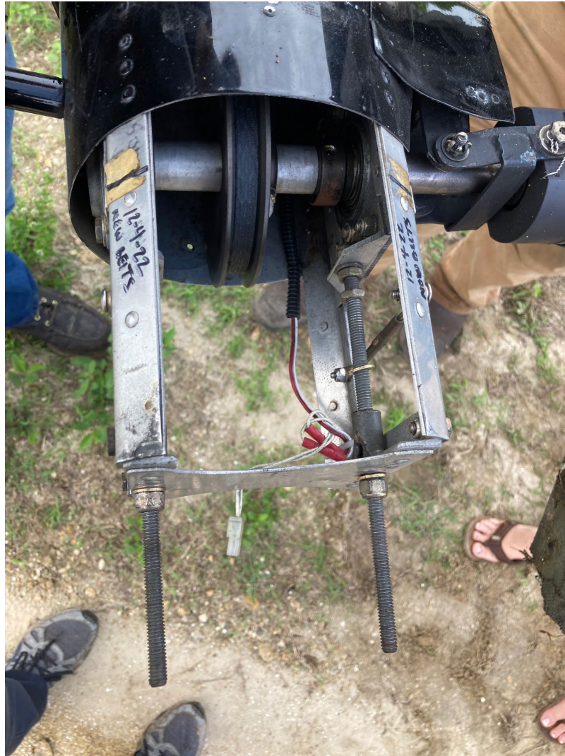
Photograph 3 - Tail rotor drive belt jam nut out of position. (Courtesy of Pilot/Owner)
