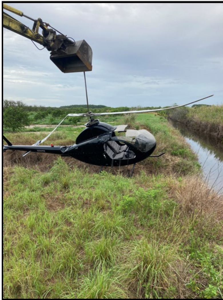
Photograph 5 - Helicopter during recovery. Note the damage to the rotor blades and tail boom. (Courtesy of Pilot/Owner)
