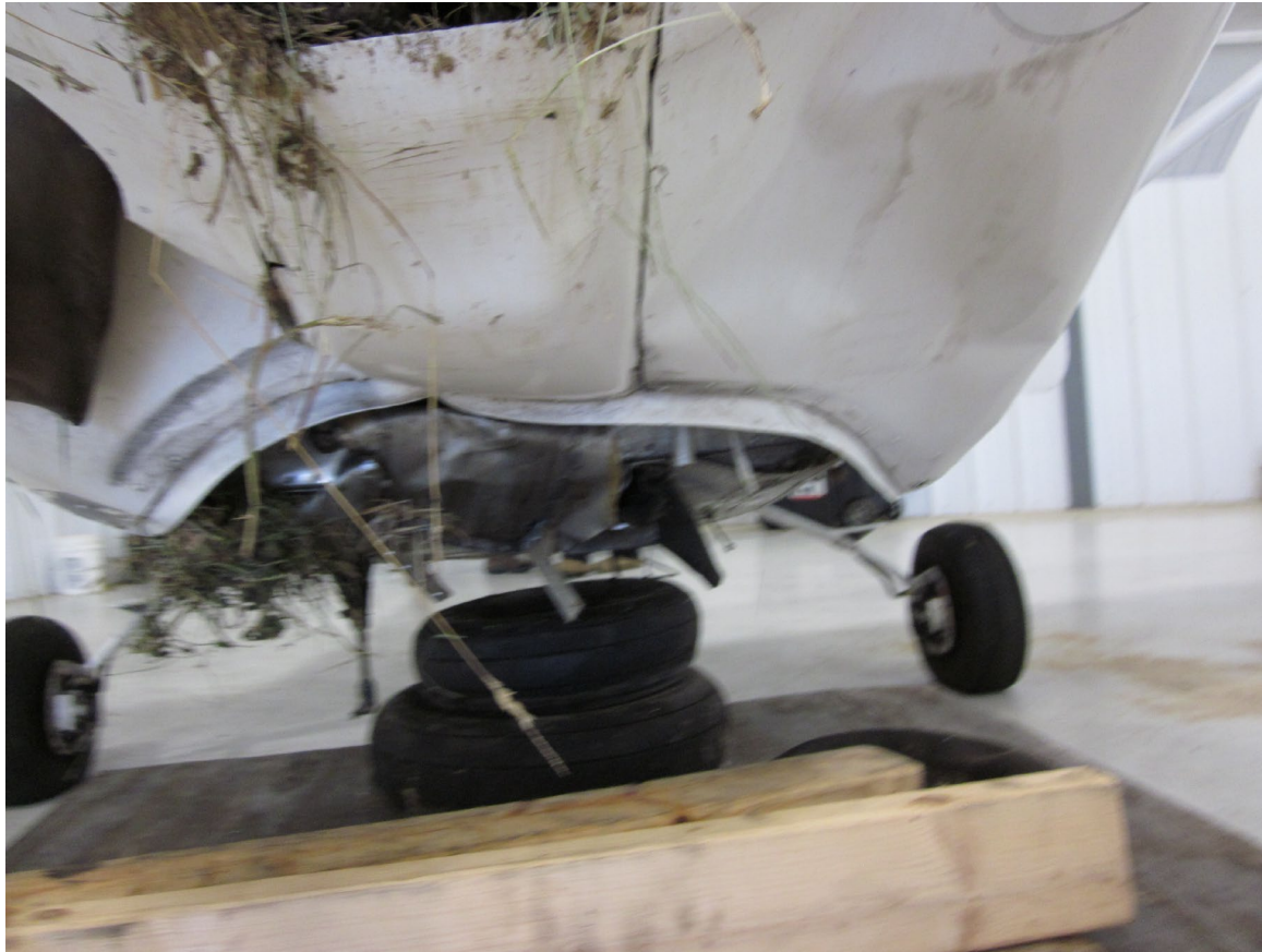
Photograph 2 - Underside of airplane showing damage to the fuselage (Courtesy of FAA)
