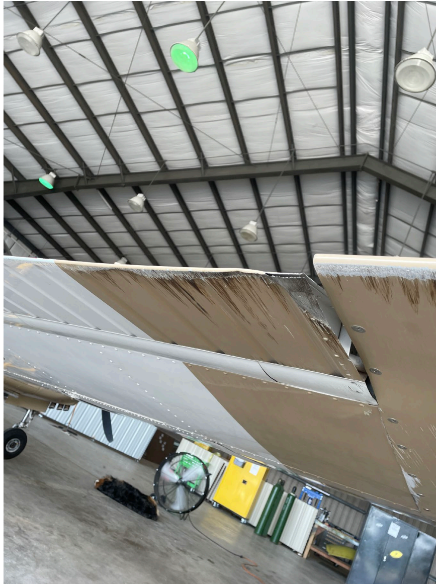
Photograph 1 - Right aileron damage (Courtesy of FAA)
