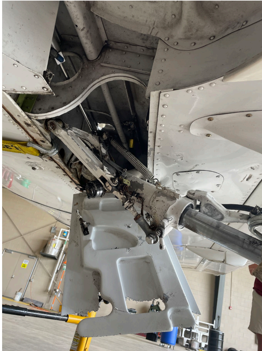
Photograph 2 - Right main landing gear collapse (Courtesy of FAA)
