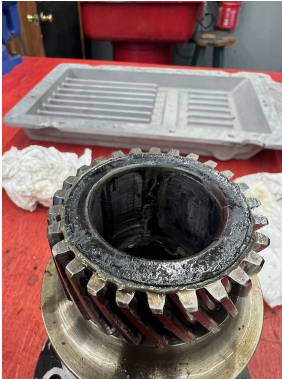
Inside of hub/gear showing sheared key. Striations on inside of hub show some non-contact areas. Hub came off with only 3 tons pressure – early hub design.
