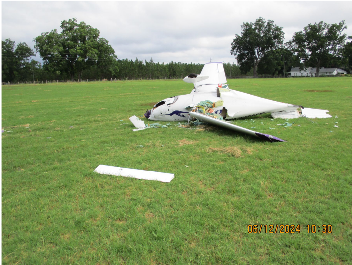
Photograph 1 - Fractures noted to fuselage and right wing (Courtesy of FAA)
