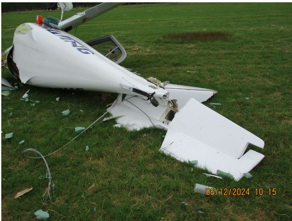
Photograph 2 - Fractures and partial separation noted to empennage (Courtesy of FAA)
