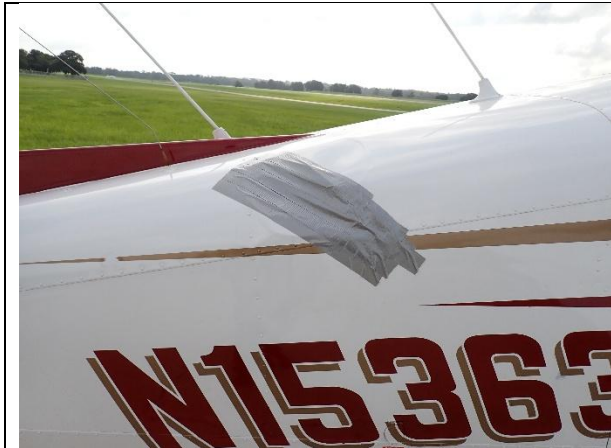
Photograph 5: Damage to fuselage (covered by tape)
