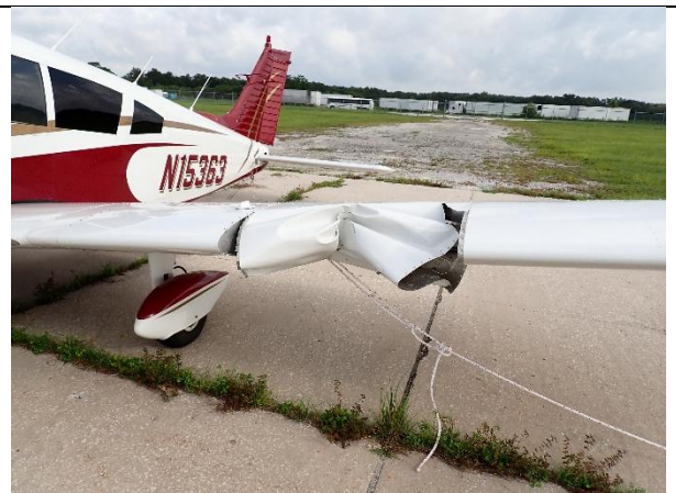
Photograph 8: Left wing with damage
