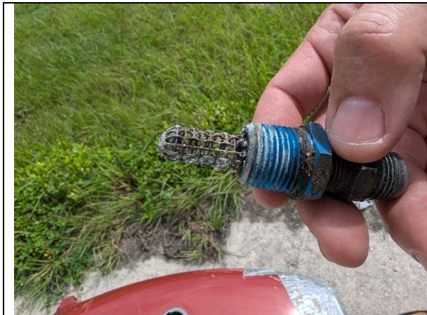
Photograph 10: Left aux tank pickup screen
