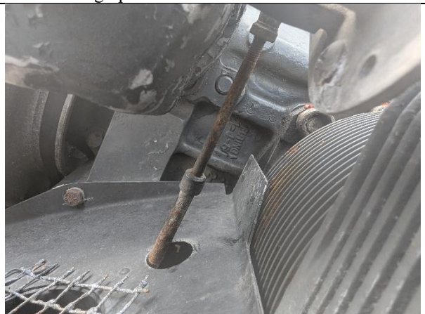
Photograph 19: Propeller governor control cable end (corroded)
