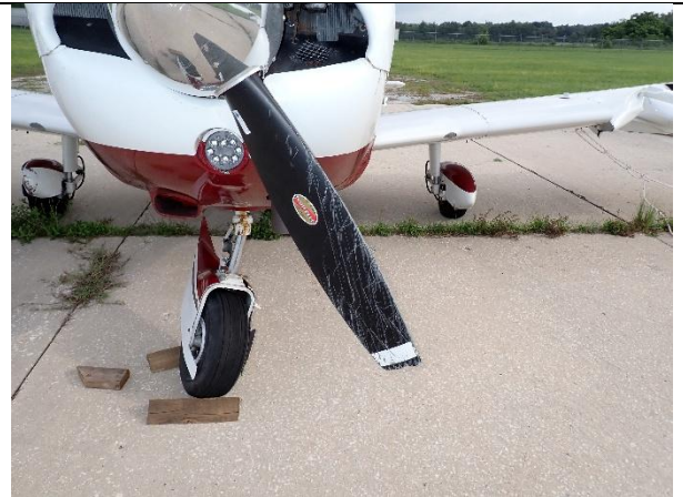
Photograph 21: Impact damaged propeller blade
