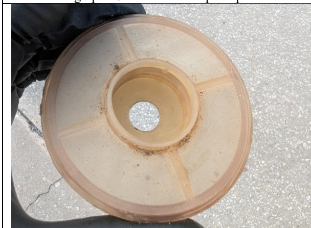
Photograph 12: Fuel strainer screen with debris in screen
