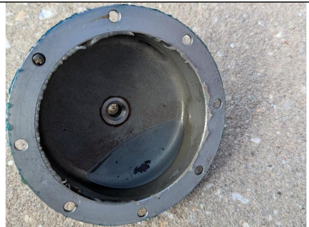
Photograph 11: Fuel strainer bowl with debris in fuel
