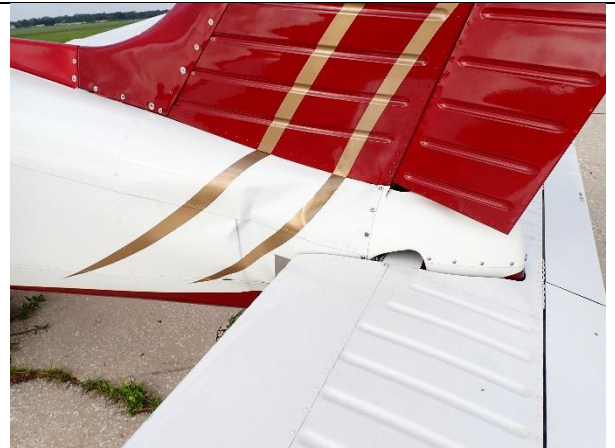
Photograph 6: Damage to empennage
