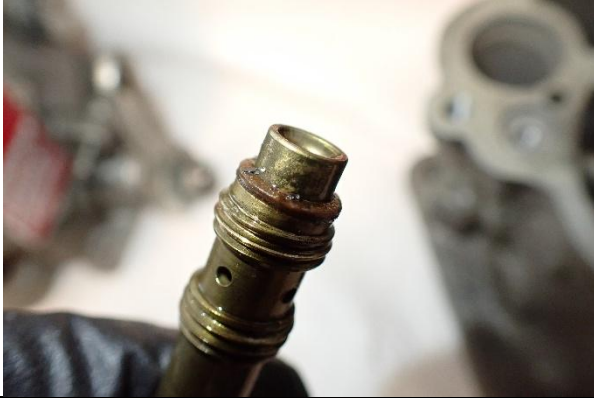
Photograph 5: Main metering jet with debris
