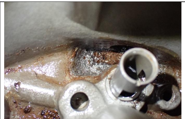
Photograph 4: Carburetor bowl with corrosion and contamination
