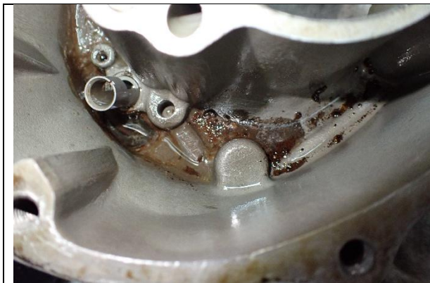
Photograph 3: Carburetor bowl with corrosion and contamination
