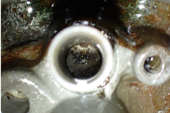
Photograph 7: Mixture control housing with debris
