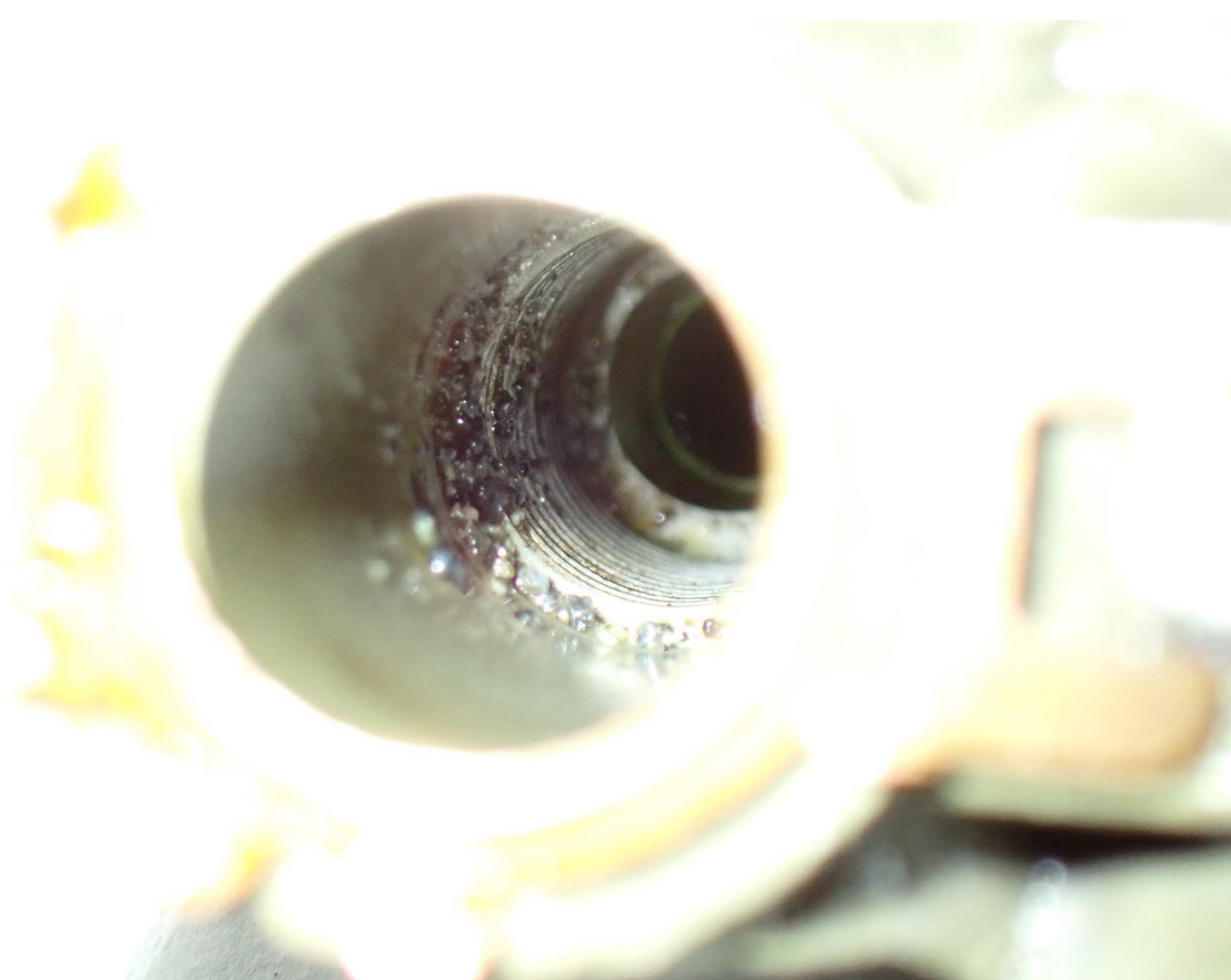
Photograph 9 - Debris found in the carburetor main metering jet well
