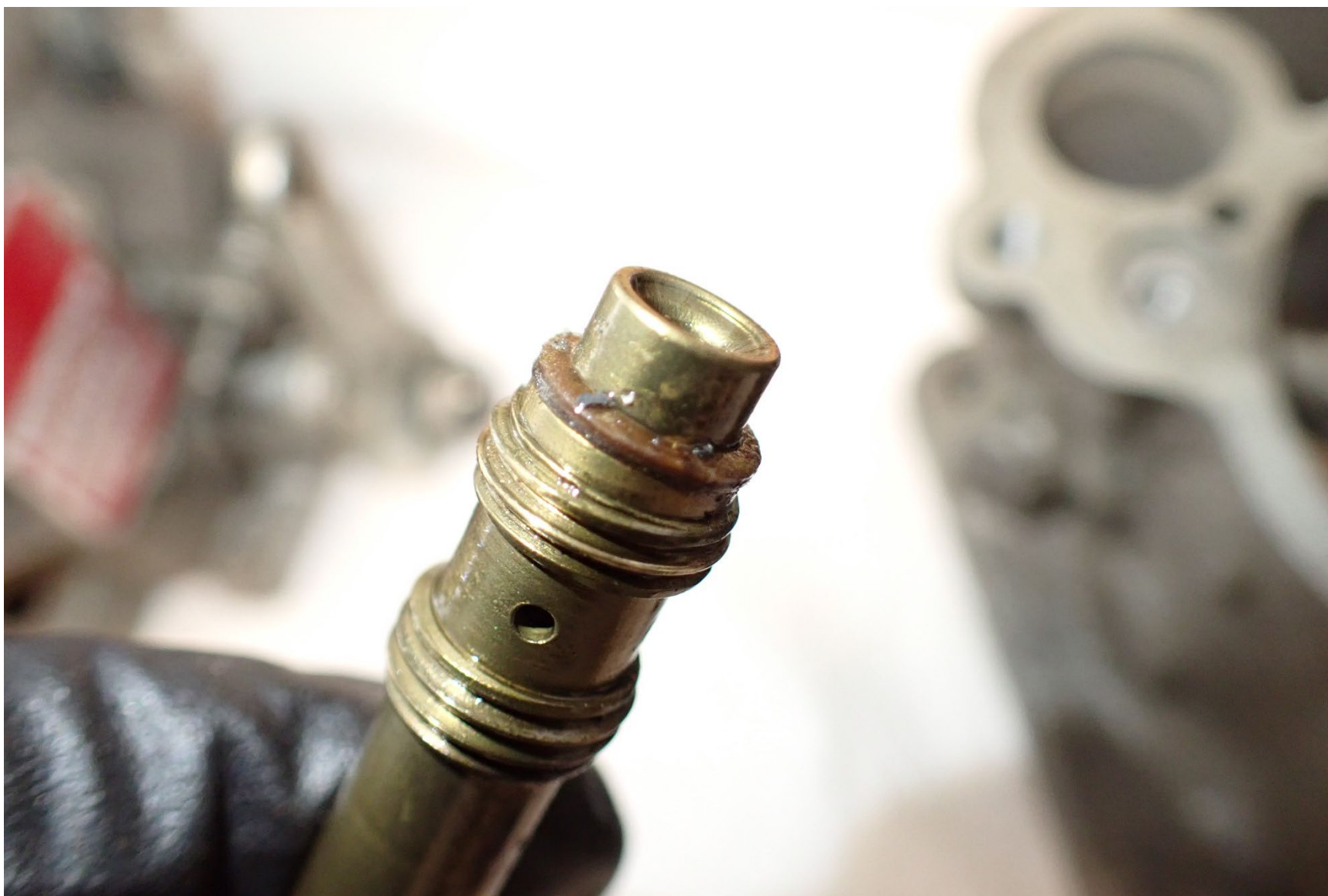
Photograph 10 - Debris found on the main metering jet
