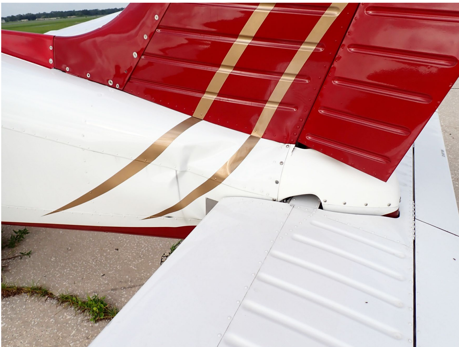
Photograph 4 - Damage to empennage
