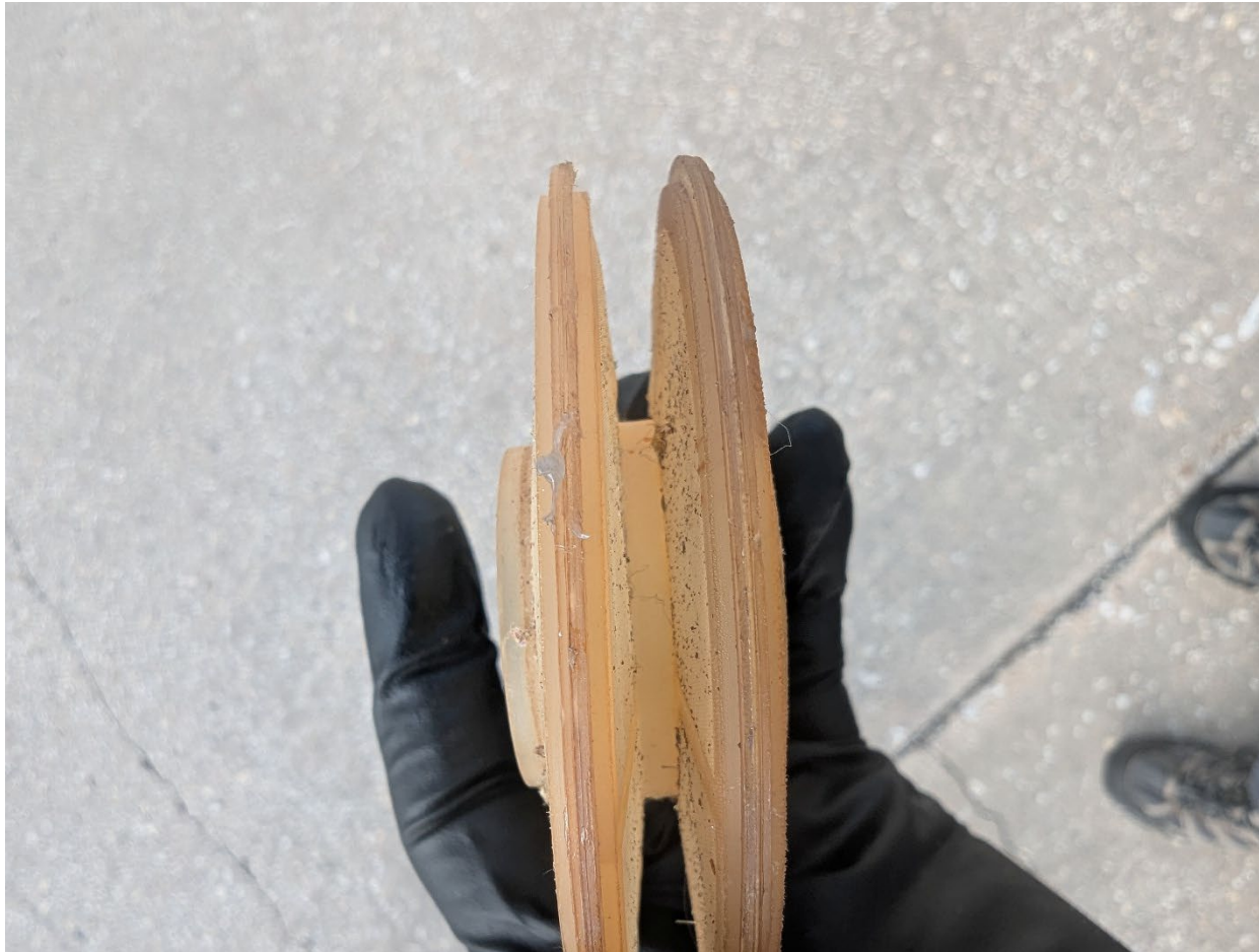
Photograph 6 - Debris found in strainer screen
