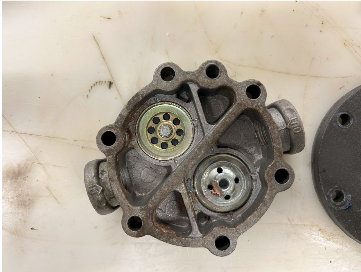
Photograph 14 - Fuel pump with corroded internal components (Source: Lycoming)
