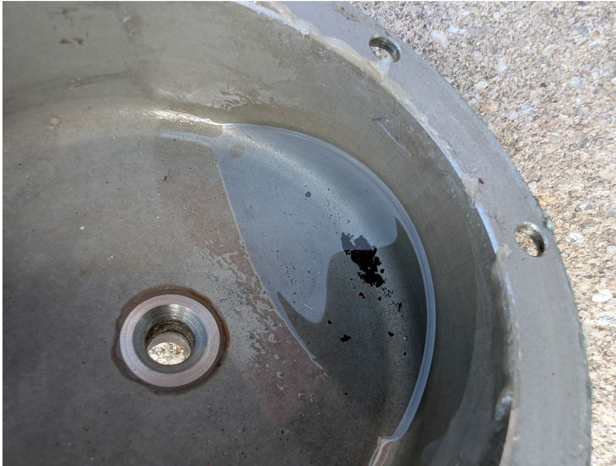
Photograph 5 - Debris found in strainer bowl
