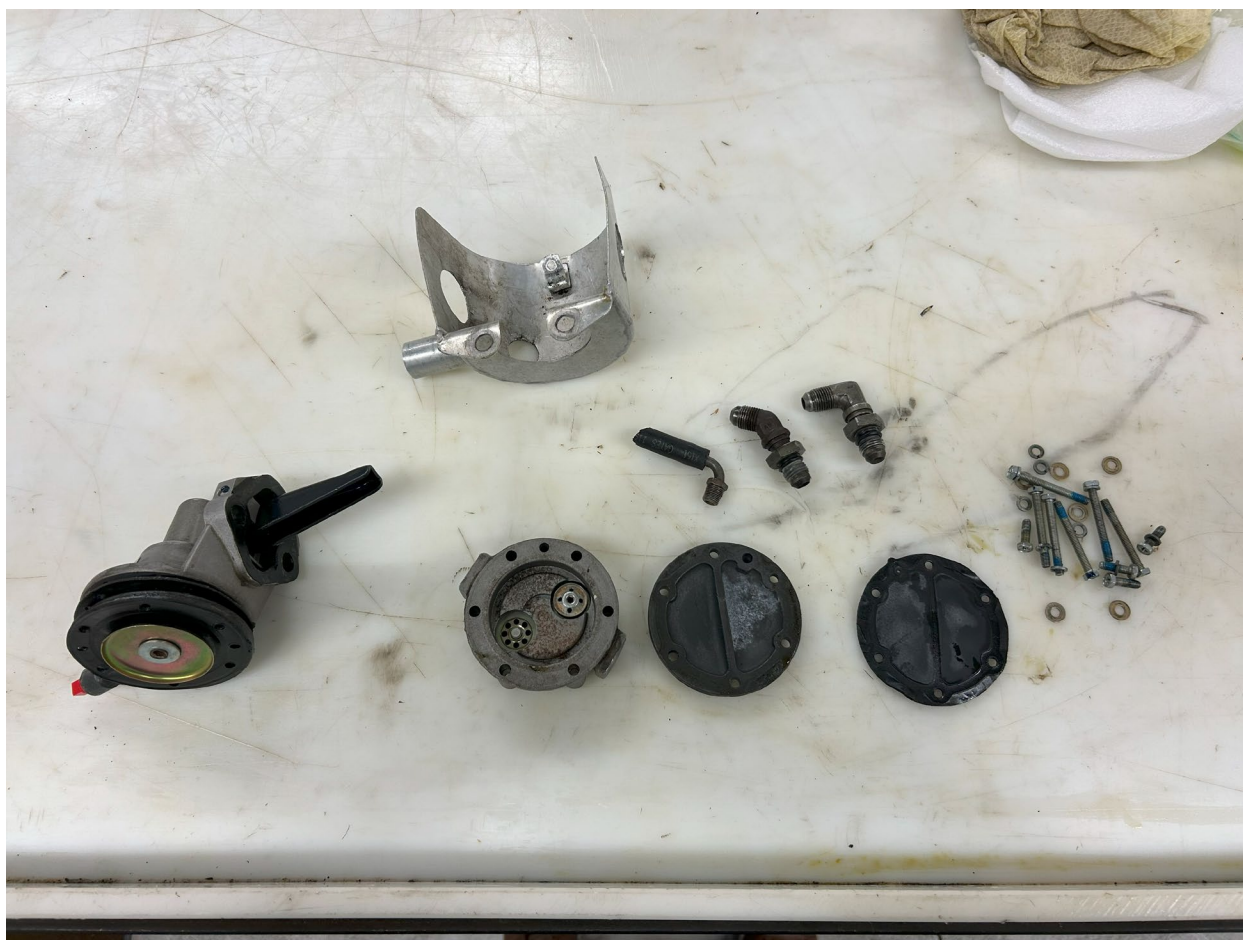
Photograph 13 - Fuel pump after disassembly
