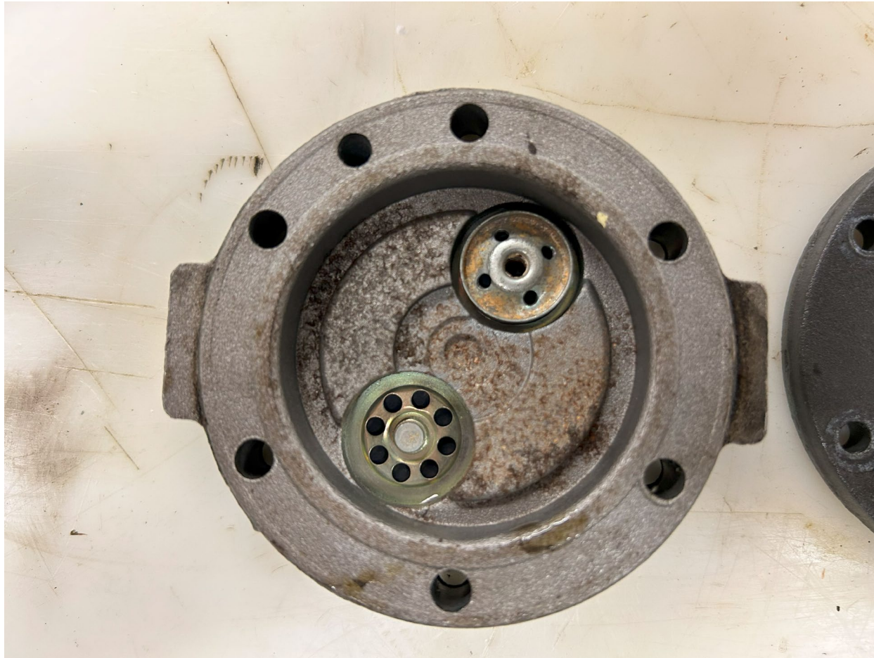
Photograph 15 - Fuel pump with corroded internal components (Source: Lycoming)
