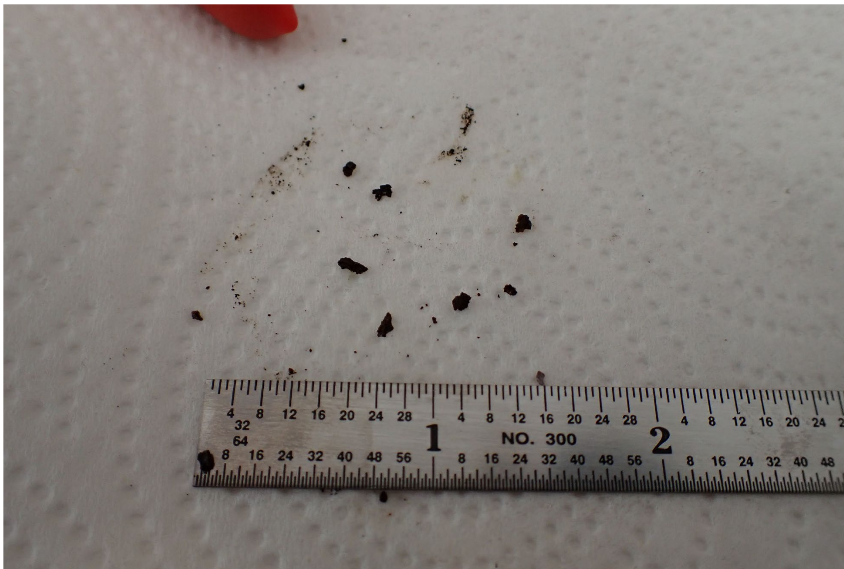
Photograph 12 - Sample of corroded debris found in the carburetor with scale
