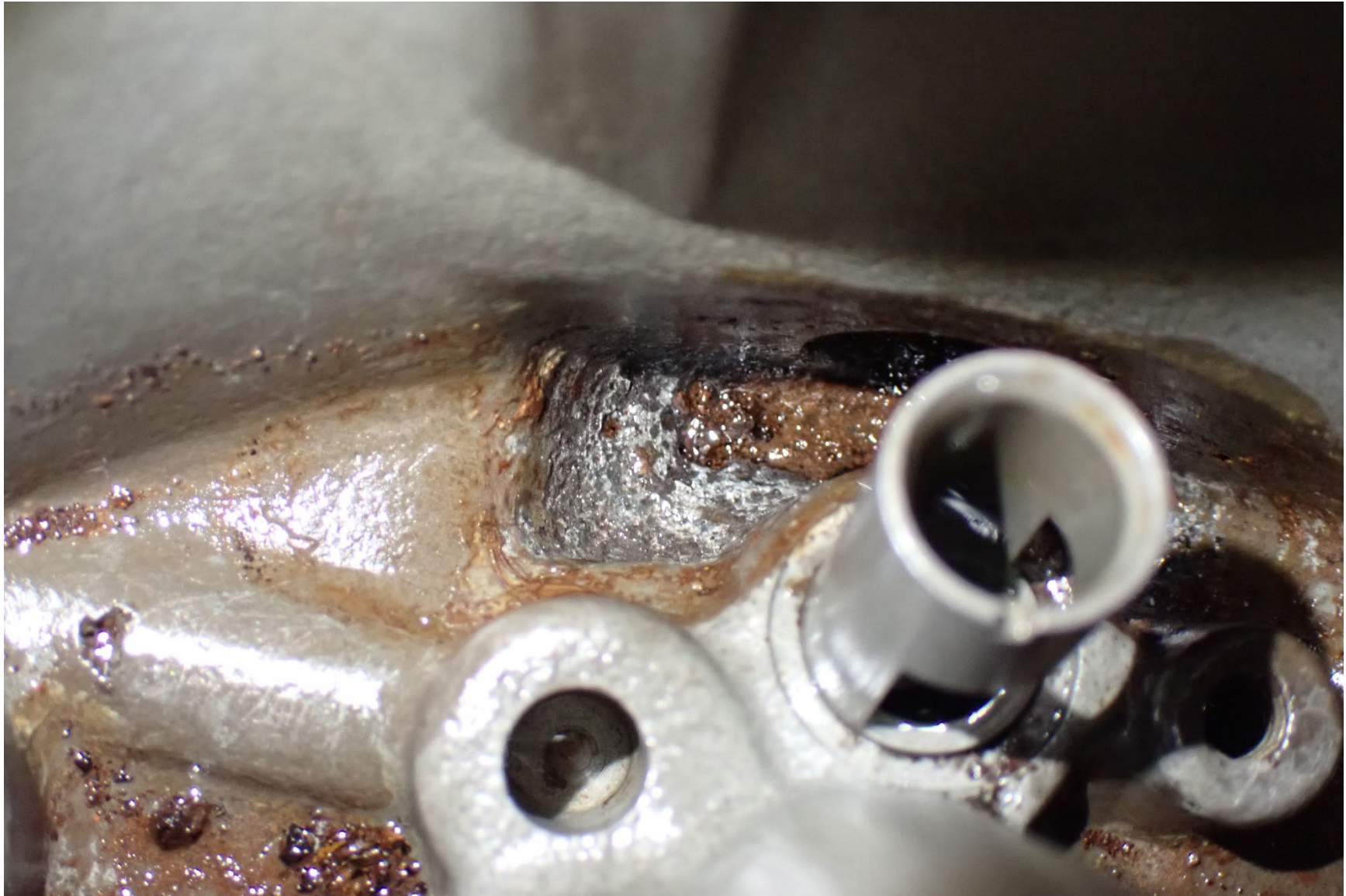
Photograph 8 - Corrosion and debris found in the carburetor bowl
