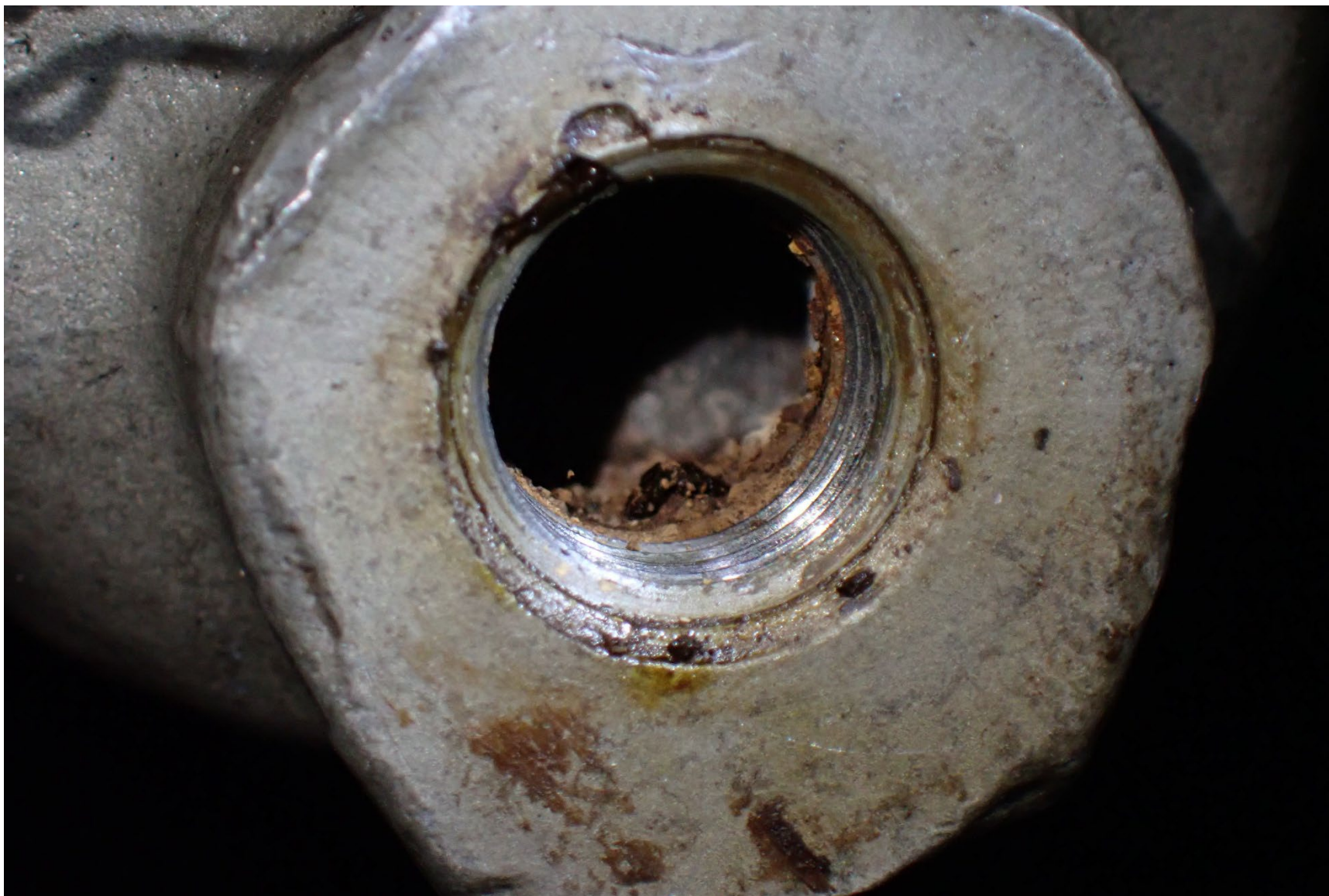
Photograph 7 - Debris found in carburetor through drain plug
