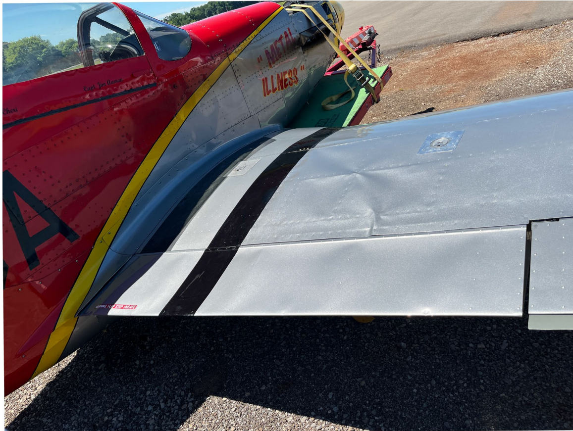
Photograph 2 - Damage to Right Wing (Courtesy of FAA)
