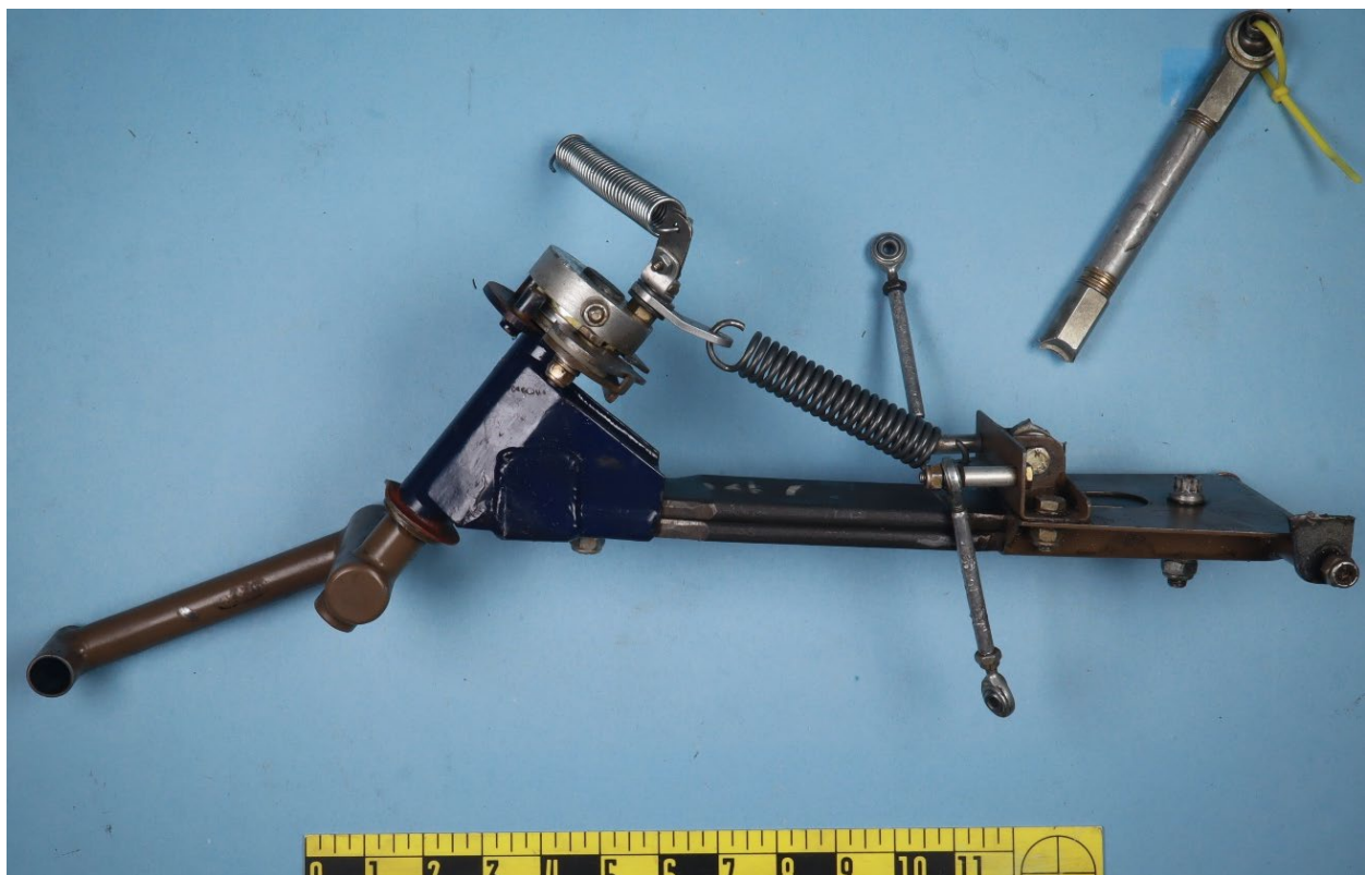
Figure 13. View of the components submitted from the tailwheel assembly.
