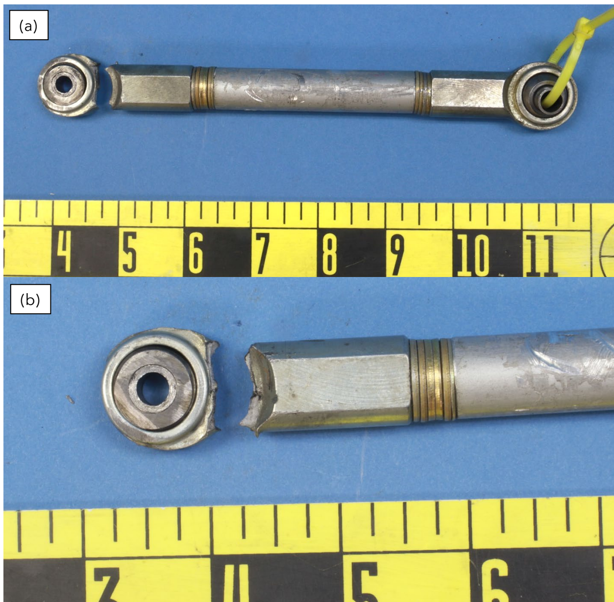
Figure 14. View of (a) the tailwheel link body and (b) a closer view of the fractured neck near the ball joint.
