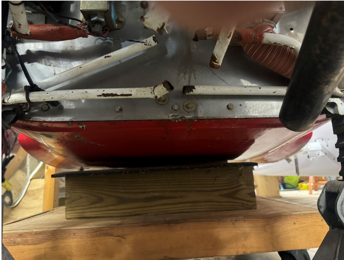
Photograph 5 - Digital Photograph From New Owner. View Showing the Broken Engine Mount Tubes
