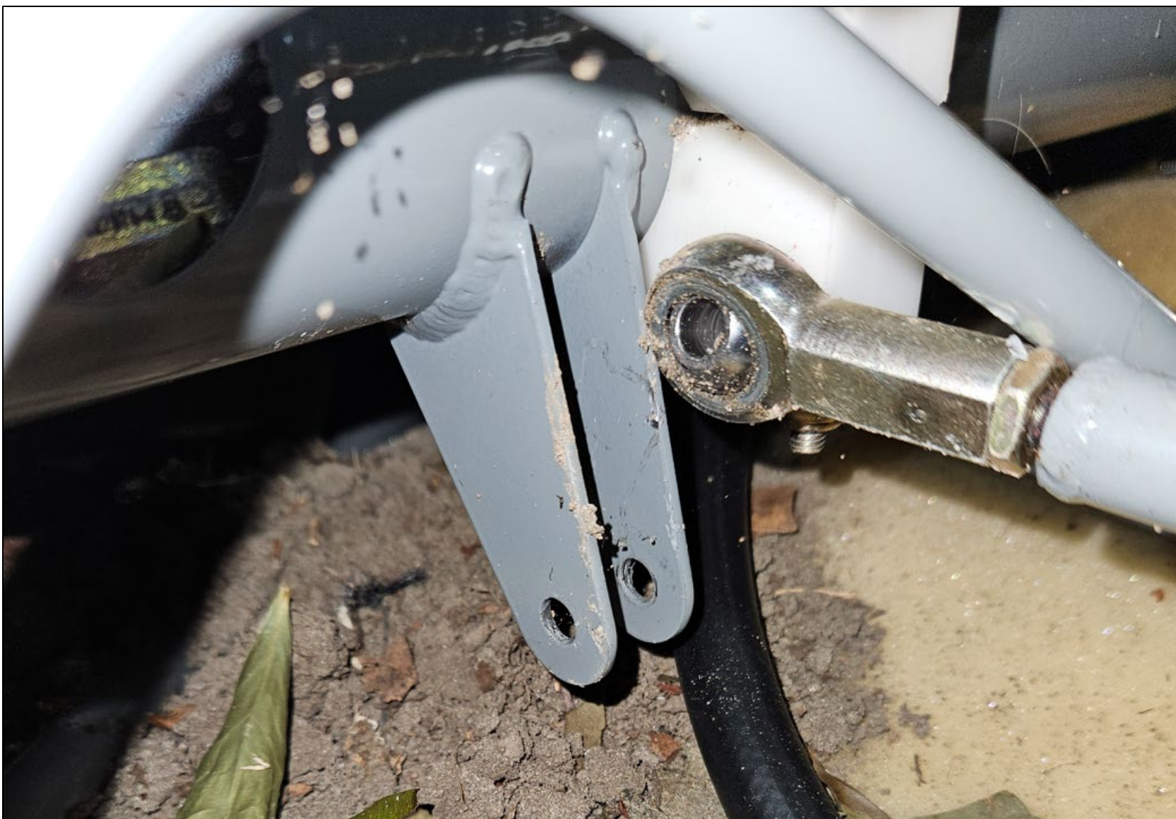
Photo 2: View of the elevator connecting rod attachment area missing its hardware (Photo Courtesy of FAA)
