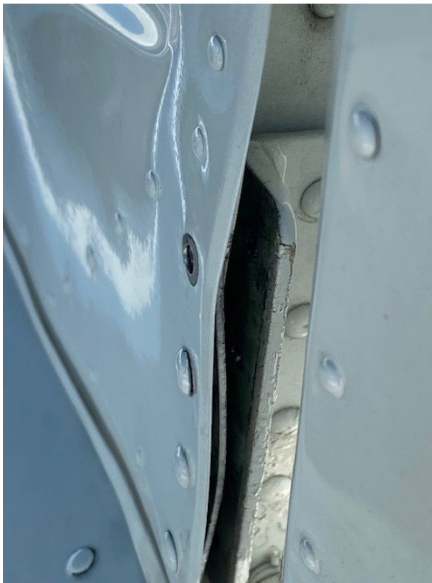
Photograph 1 - Left side vertical stabilizer with missing rivet (Courtesy of Skyborne)
