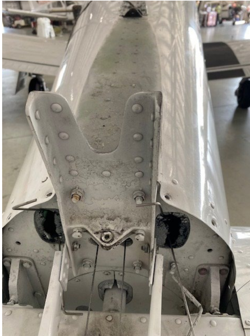
Photograph 3 - Aft mounting bracket, 17 fractured rivets (Courtesy of Skyborne)
