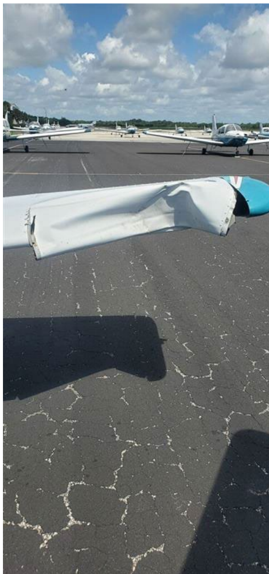
Photograph 1 - Left Wing Leading Edge Damage (Courtesy of Flight School)
