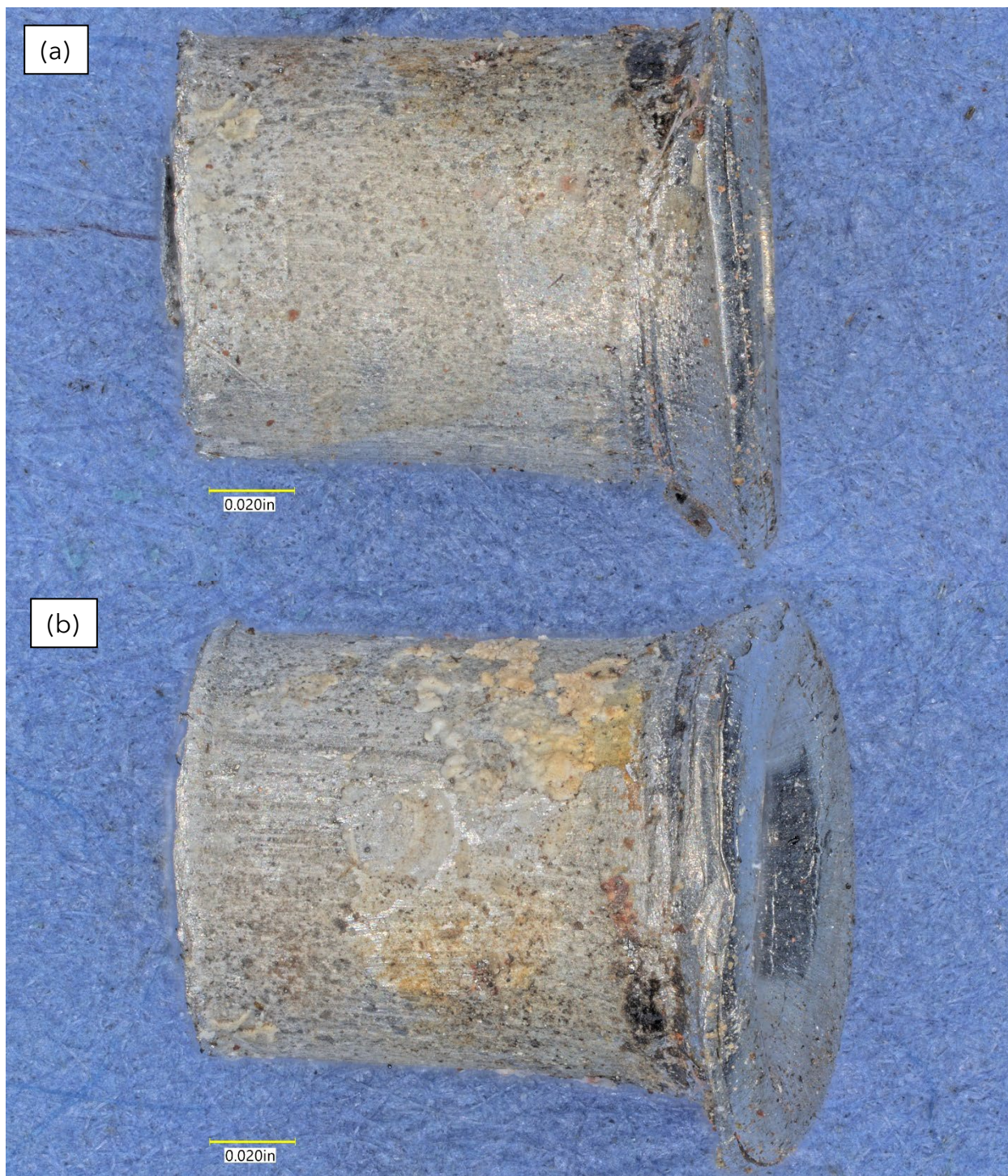
Figure 10. Opposite 180° views of the upper rivet fragment, after removal from the valve stem flange.
