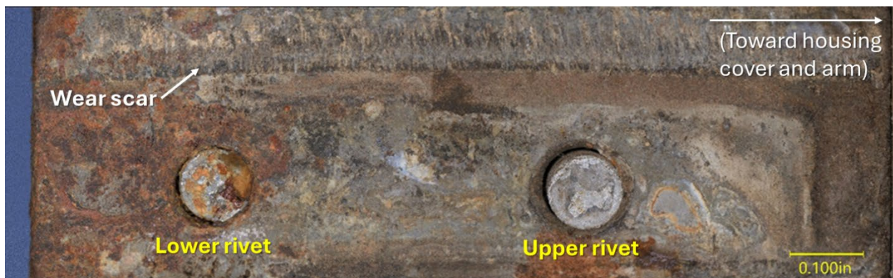
Figure 6. Closer view of the fractured rivets from the valve stem flange, showing a horizontal streak of sliding wear.
