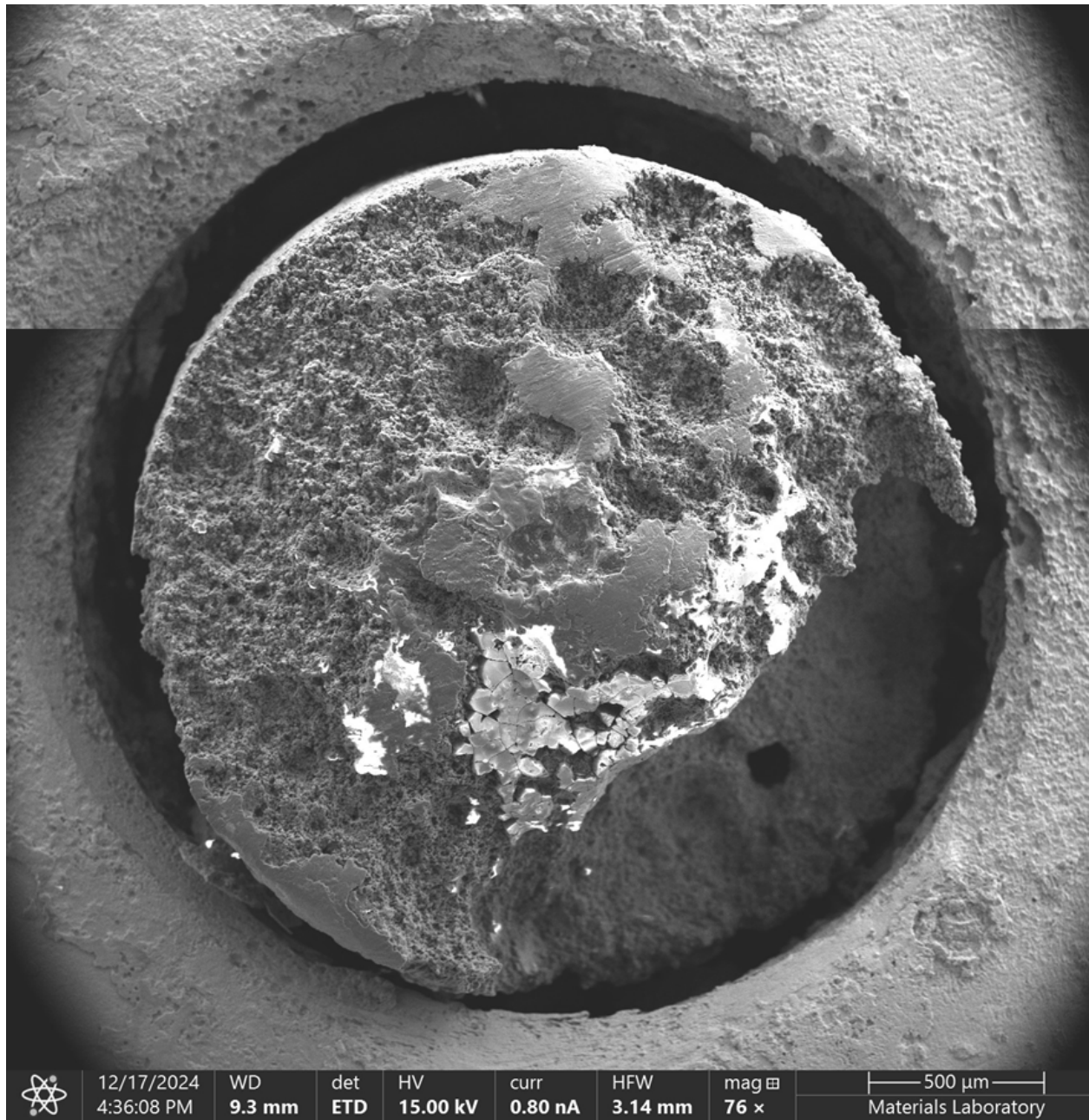
Figure 16. SE montage image of the lower rivet fracture surface.
