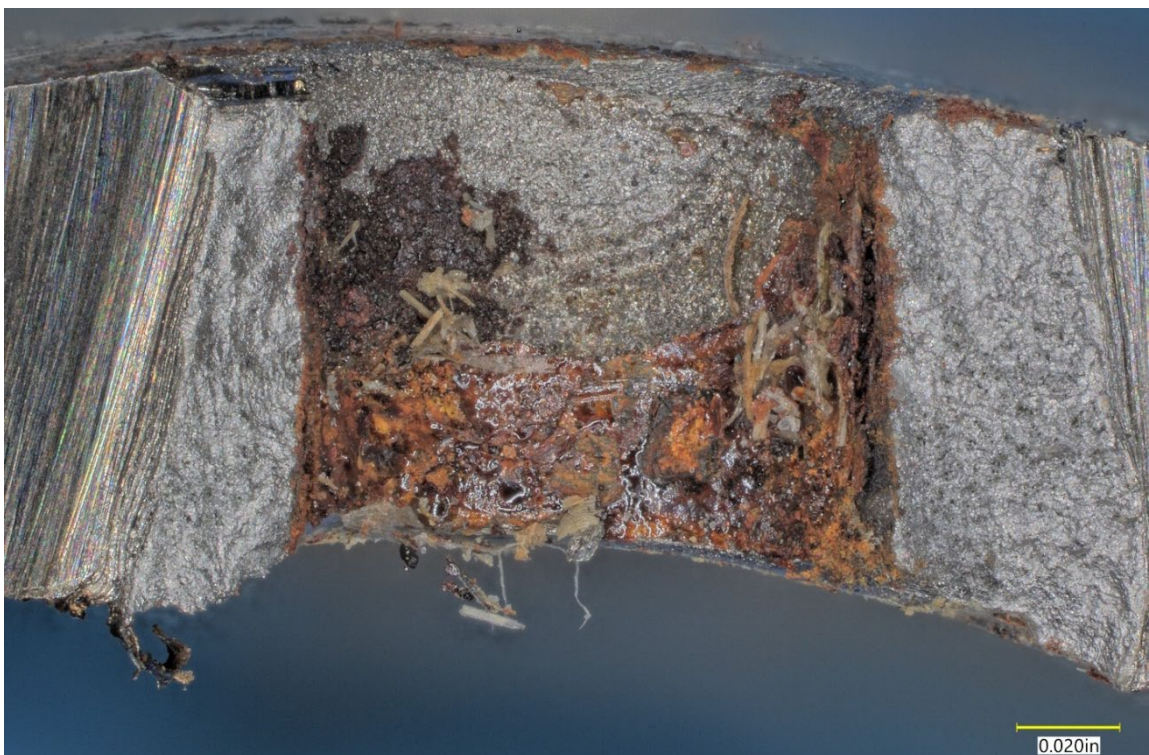
Figure 22. Sectioned and opened rivet hole at the location of the lower rivet.
