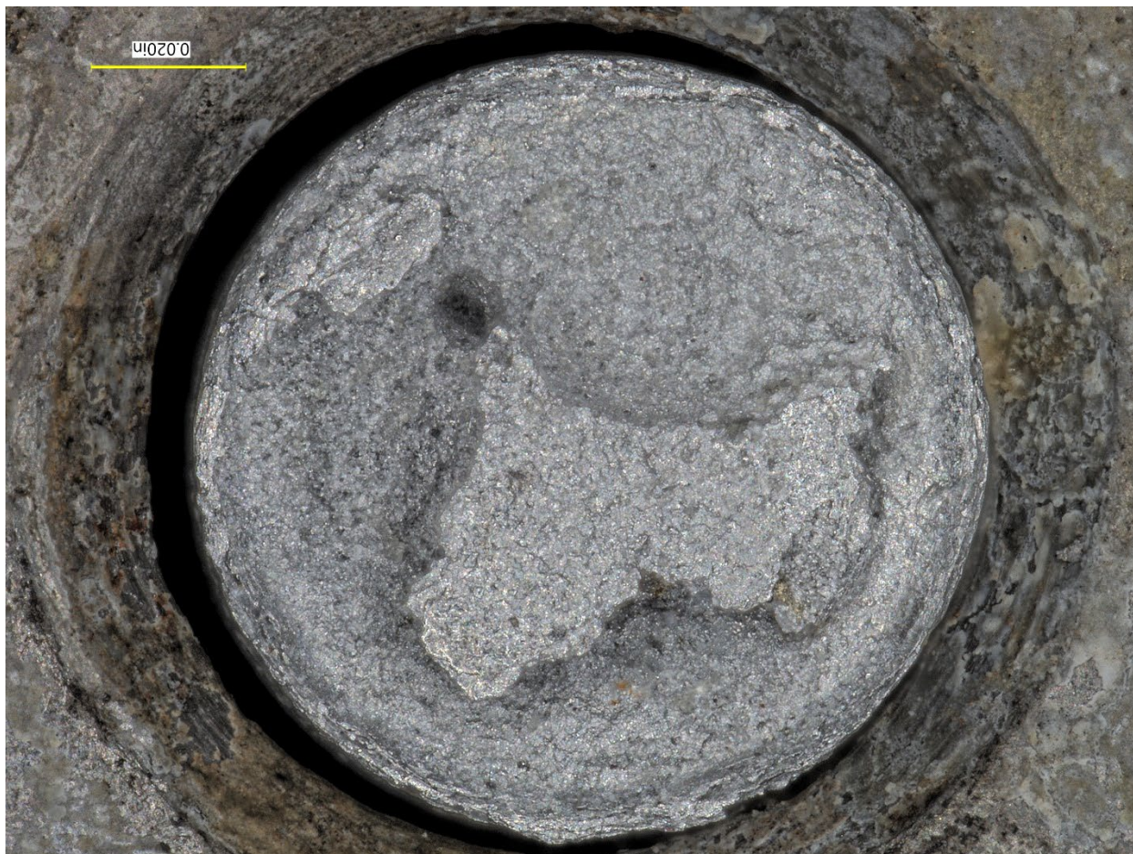
Figure 8. View of the upper rivet, after cleaning.
