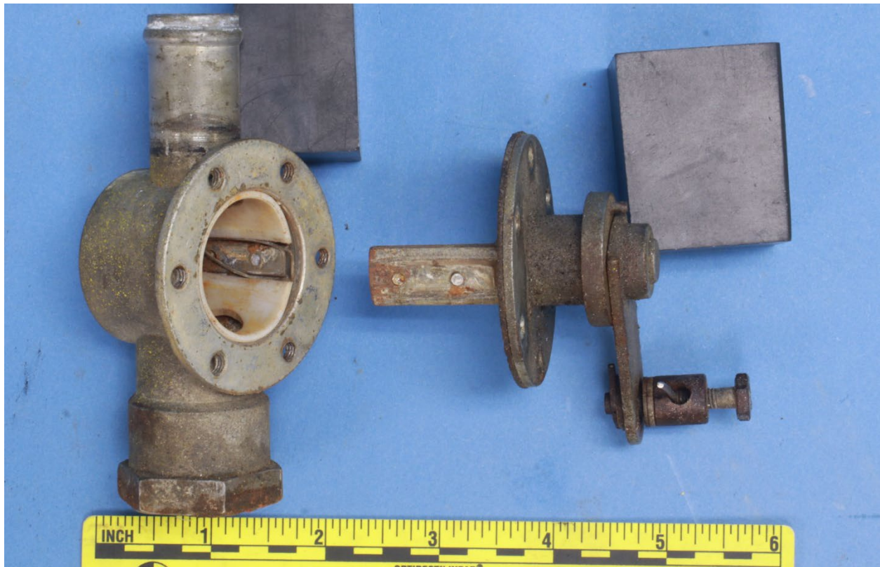
Figure 3. View of the valve body and stem positioned showing the rivet fracture surfaces.
