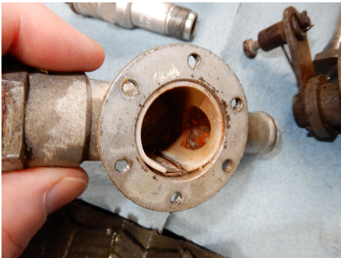
Photograph 7 - Fuel Shutoff Valve (NTSB Photo)
