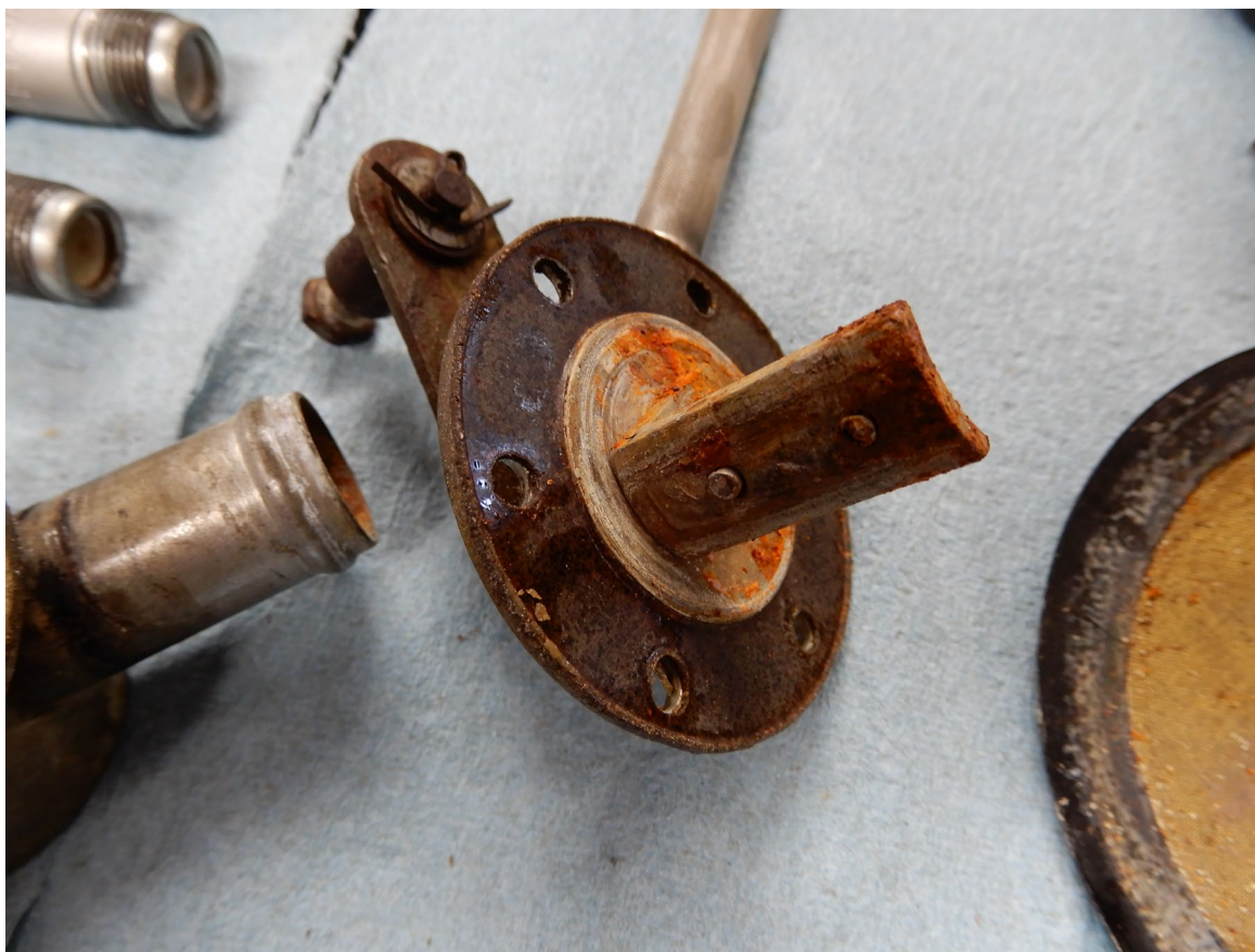
Photograph 8 - Fuel Shutoff Valve (NTSB Photo)
