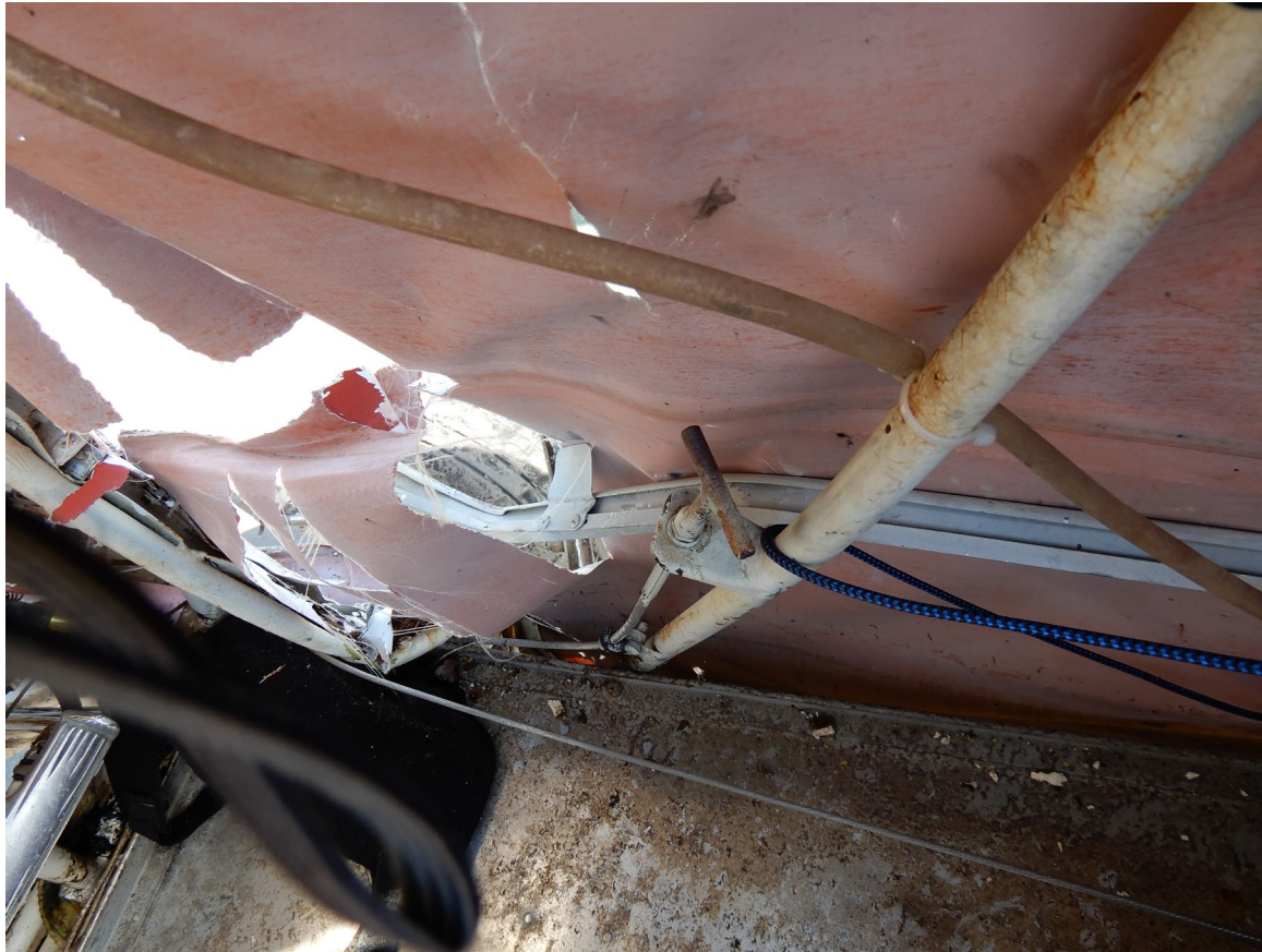
Photograph 5 - Fuel Shutoff T-Handle (NTSB Photo)
