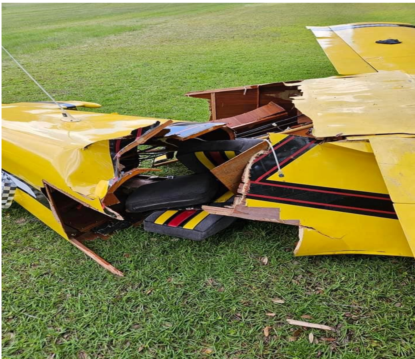
Photograph 2 - View of fuselage damage. (Courtesy of FAA)
