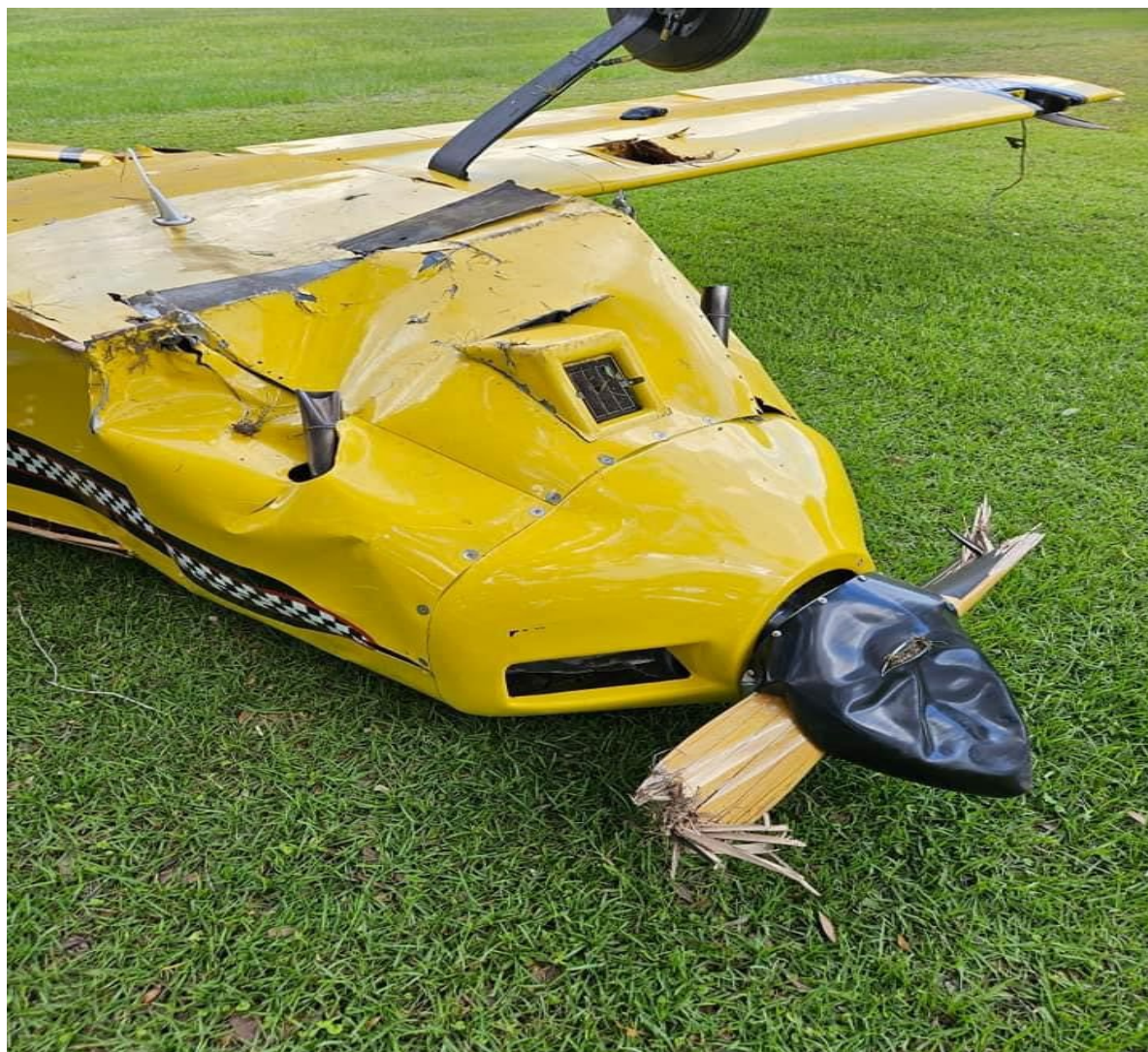
Photograph 1 - View of nose of airplane inverted showing wing and fuselage damage. (Courtesy of FAA)
