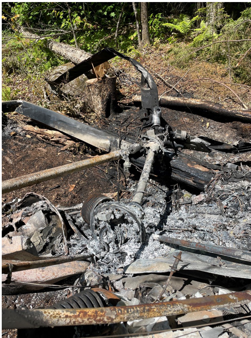
Photograph 3 - Main rotor assembly and drive shaft (Courtesy of FAA)
