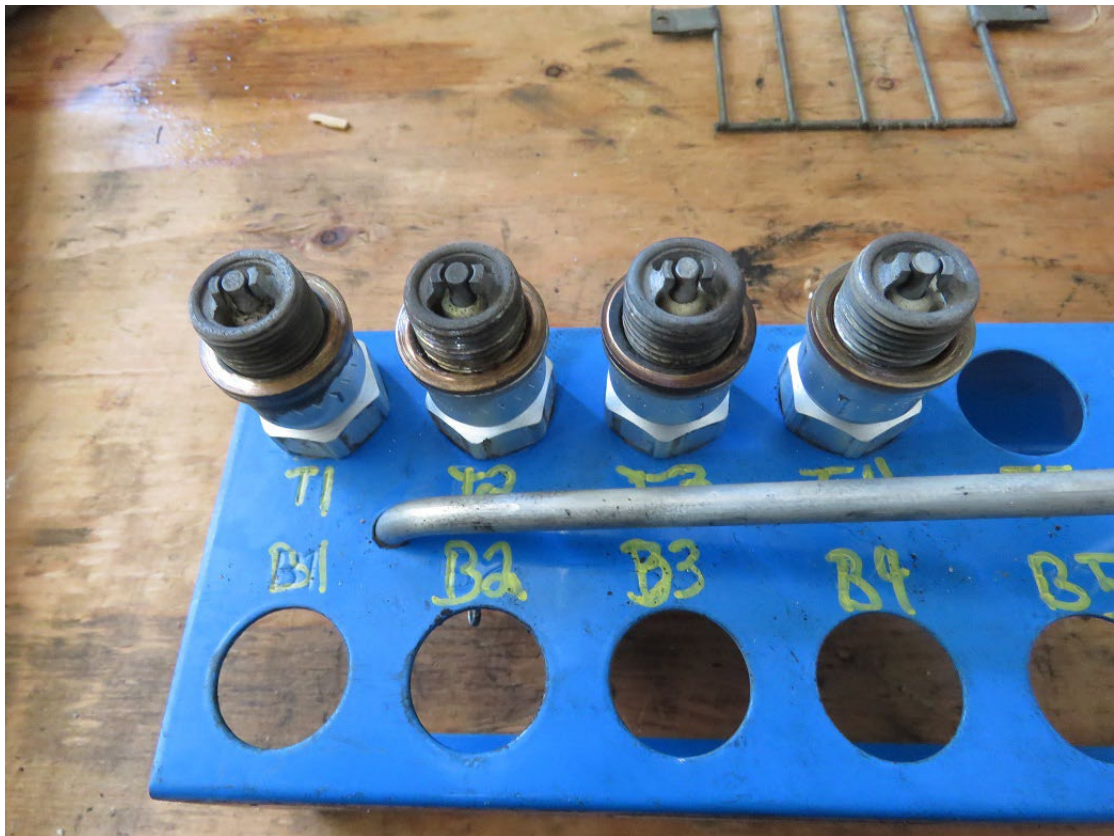
Figure 3 - Top Spark Plugs, Removed from Cylinders (Courtesy of Lycoming)
