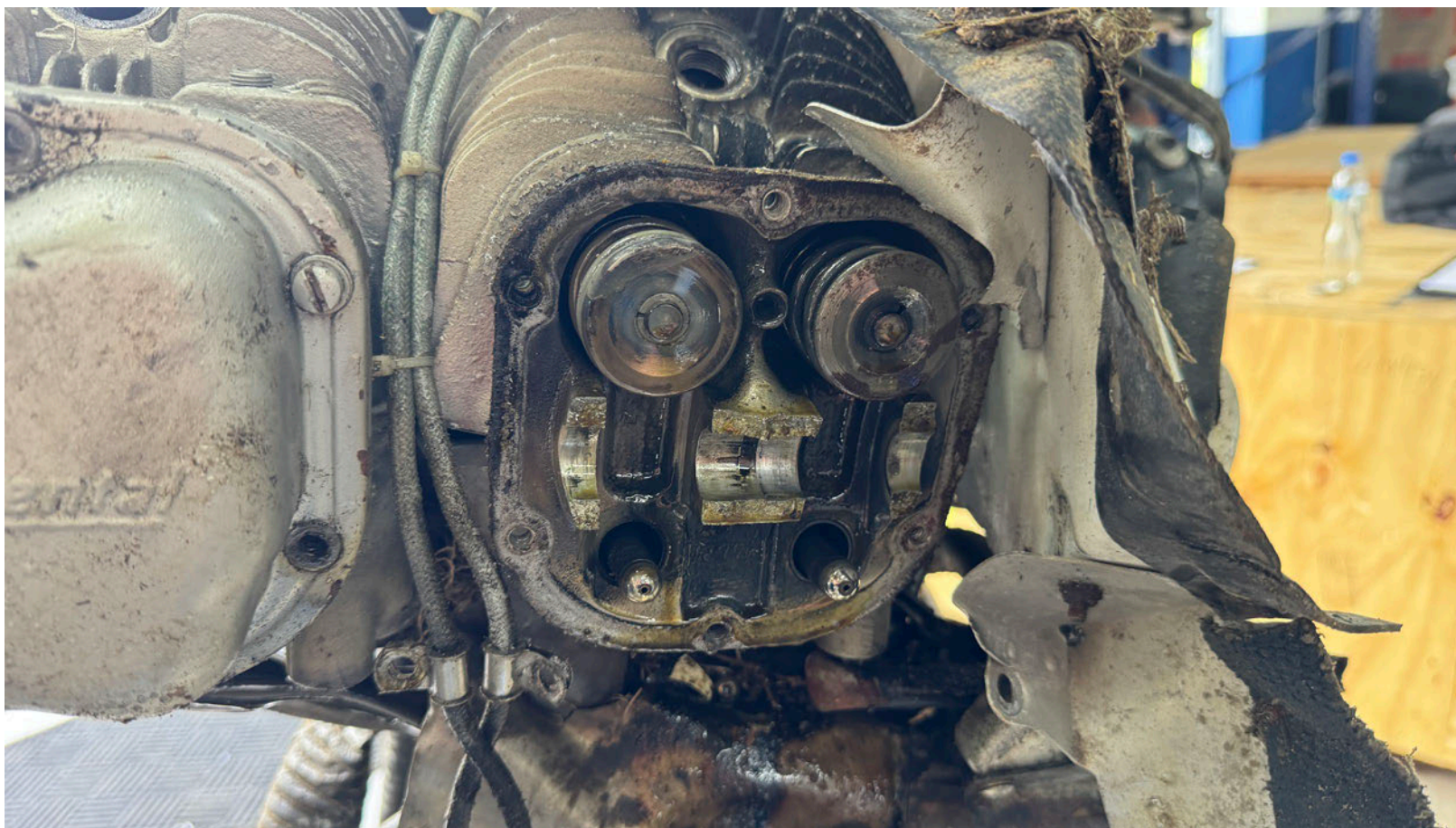
Photograph 6 - View of the No. 2 Cylinder with rocker box cover removed. (Courtesy of FAA)
