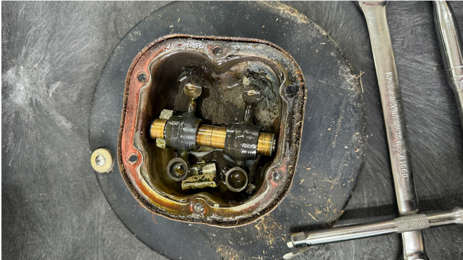
Photograph 5 - View of the No. 2 cylinder rocker box cover with fractured parts. (Courtesy of FAA)
