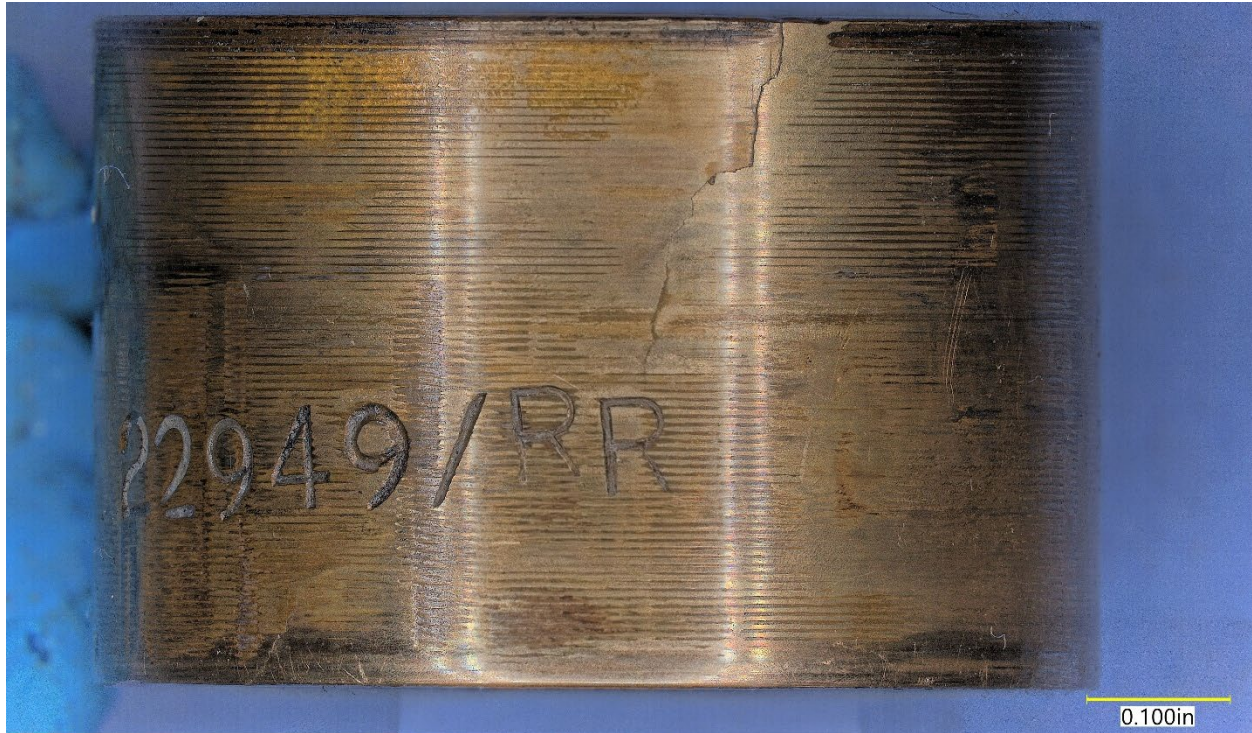
Figure 10. The outside diameter surface of the right bushing from the shaft in Figure 8.
