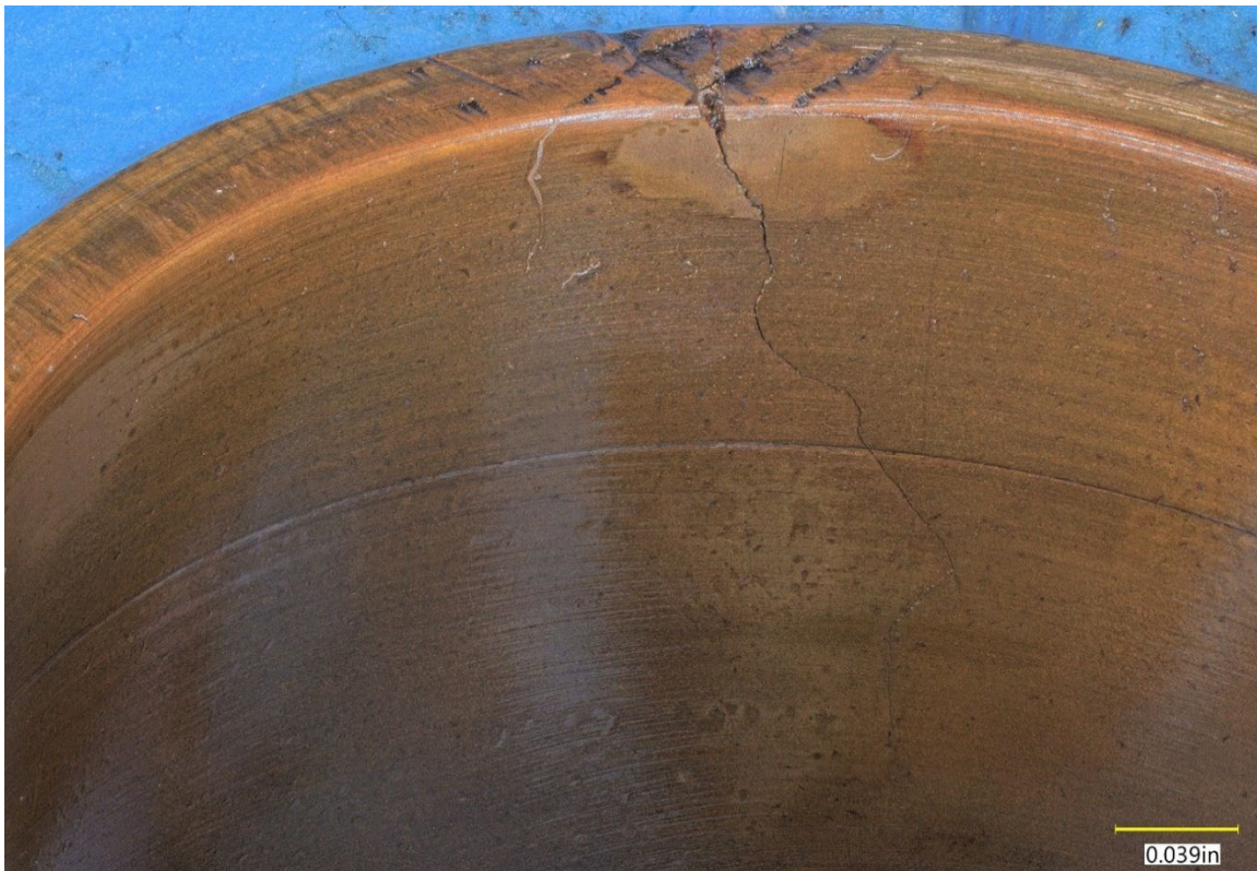
Figure 11. Angled inside diameter view of the right bushing, showing an ovoid wear depression and crack emanating from the edge.
