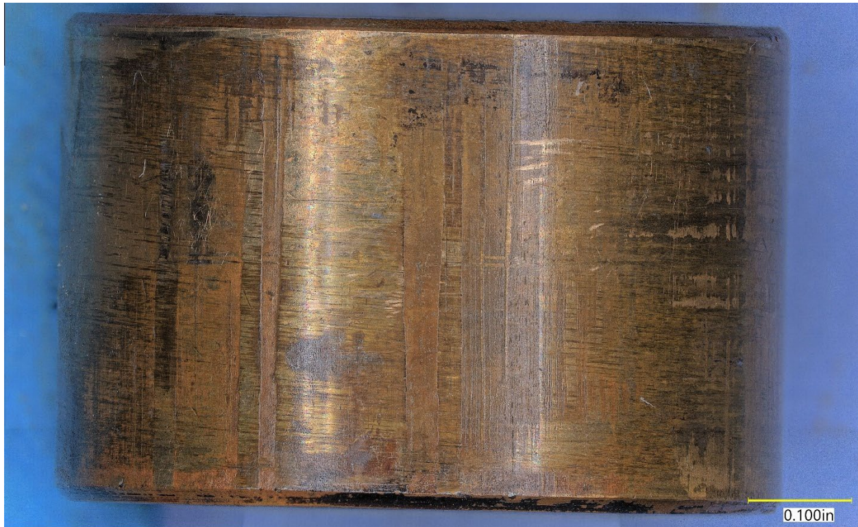
Figure 12. Outside diameter of the left shaft bushing from Figure 8.
