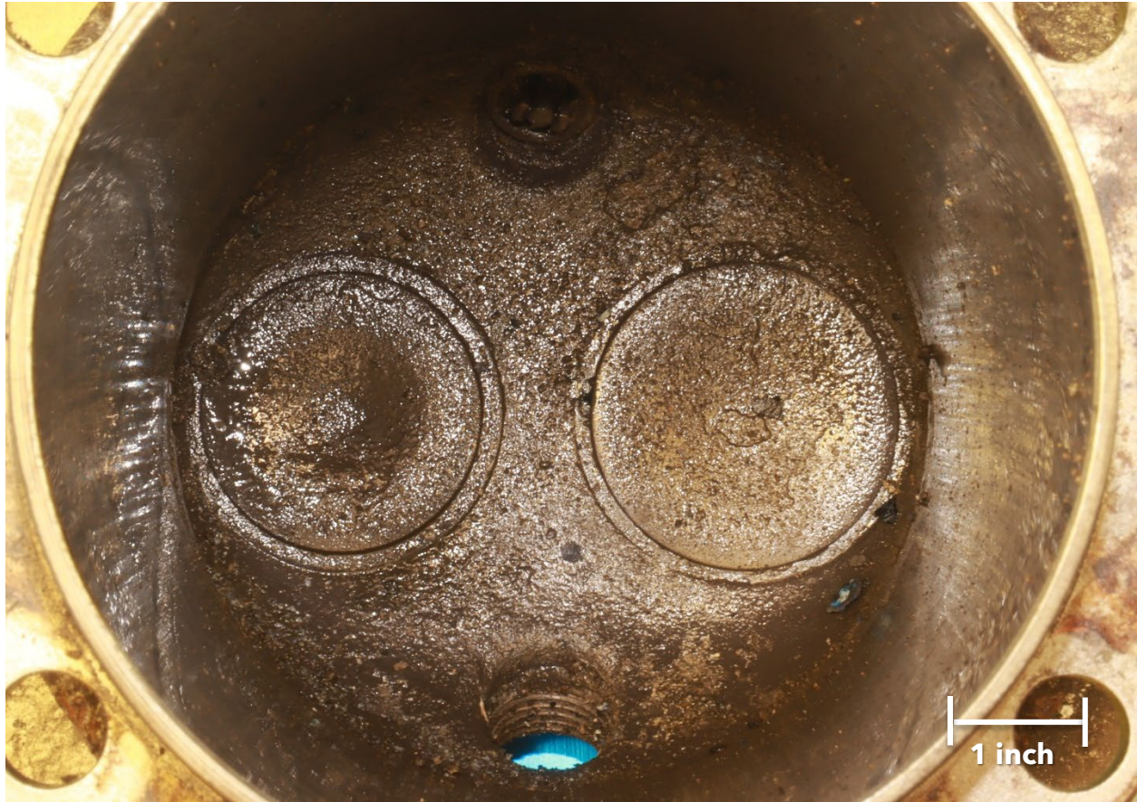
Figure 3. View of the cylinder interior, as received, showing the two valve heads.
