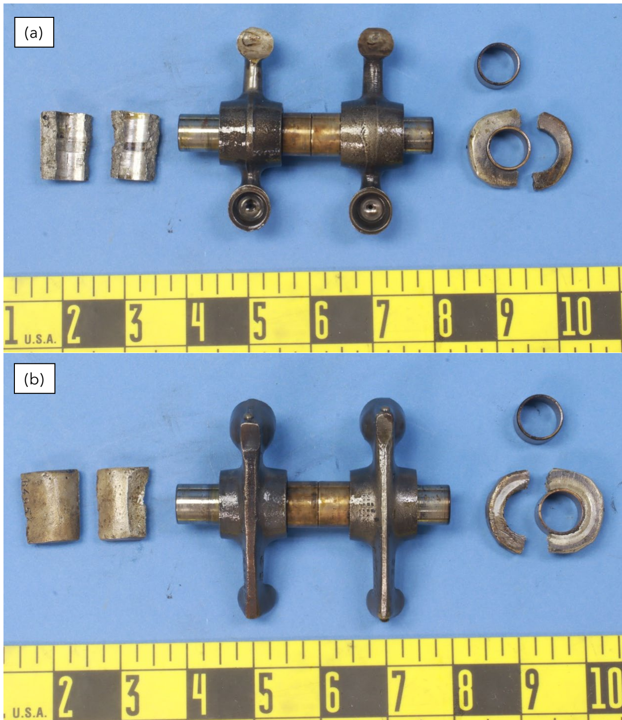
Figure 5. View of the rocker arms and bushing on the shaft, with fractured and separated pieces of the housing, viewed from opposite sides.
