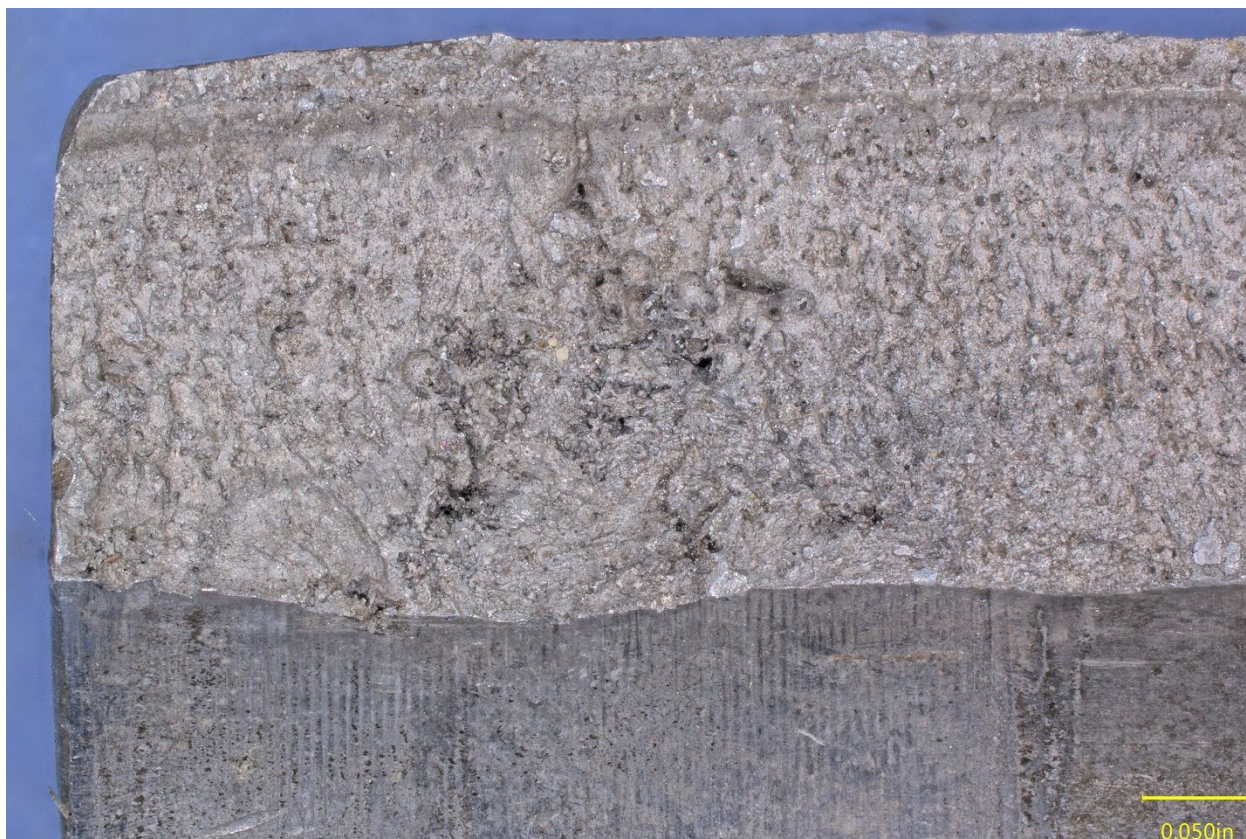
Figure 18. Left side of the center boss fragment fracture surface.
