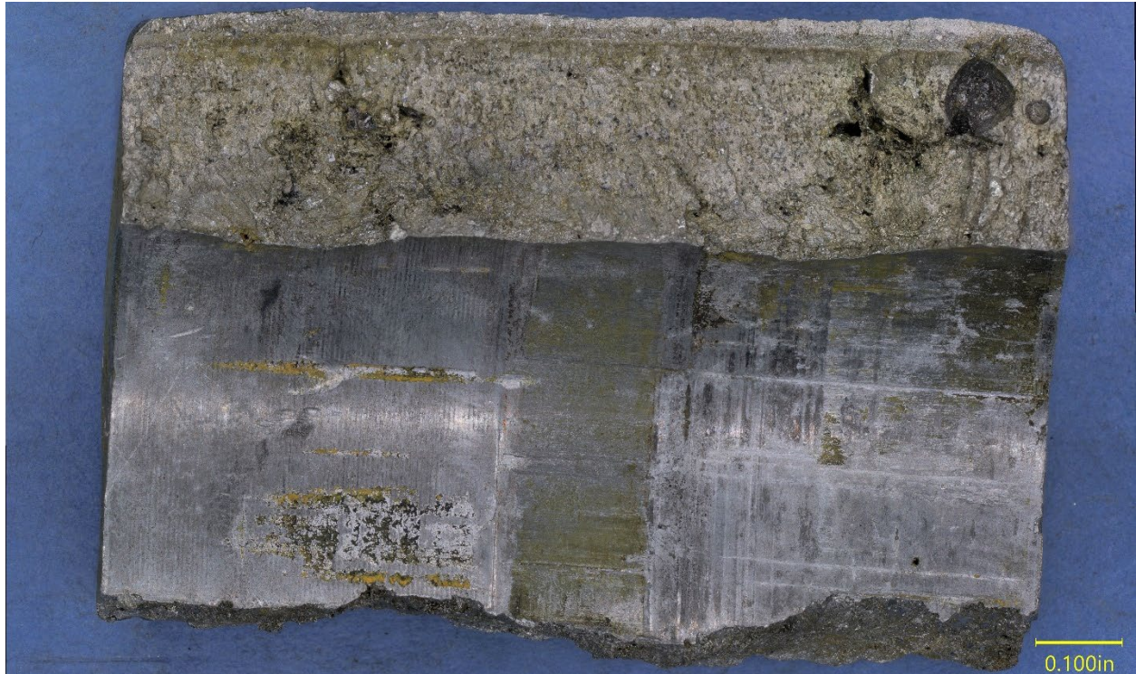
Figure 16. Overall view of the flat fracture surface on the center boss fragment.
