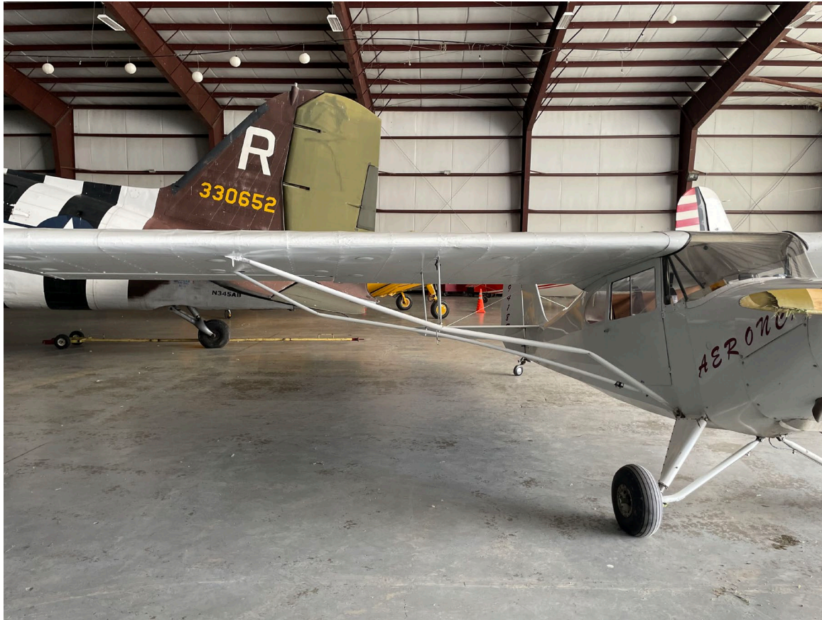
Photograph 2 - FAA Digital Photograph. Right Quartering View of the Right Side of the Fuselage and Portion of Right Wing. Note both Wing Lift Struts damaged
