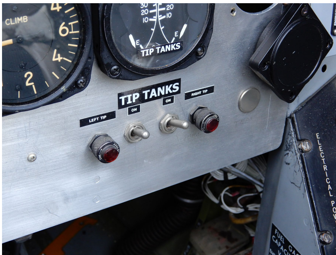
Photograph 4 - Tip Tank Switches and Lights (NTSB Photo)
