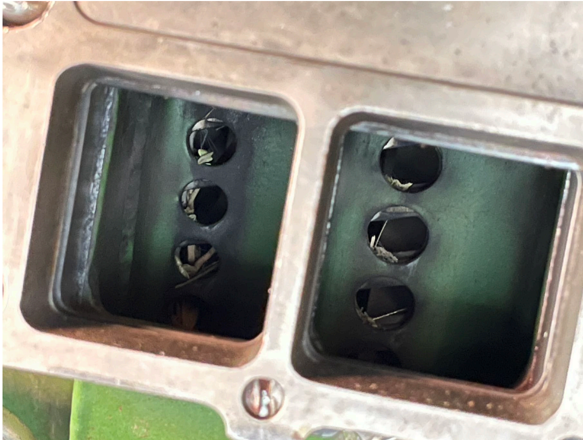
Photograph 9 - Compressor Bleed Valve Holes (NTSB Photo)
