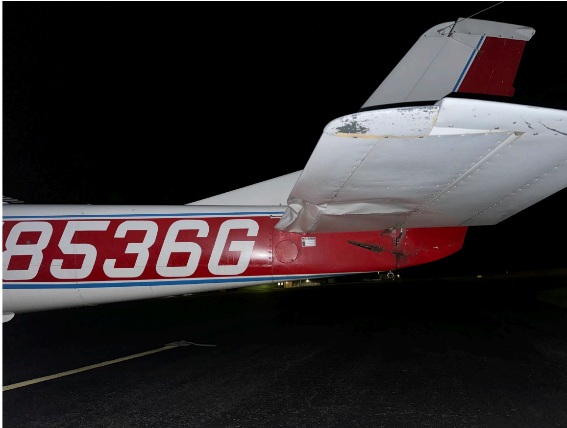
Photograph 1 - View of left horizontal stabilizer showing leading edge damage (Courtesy of FAA)
