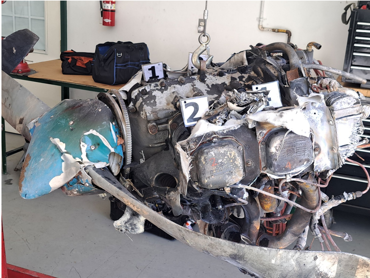
Photograph 6 - View of number 2 and 4 side of engine. (NTSB)
