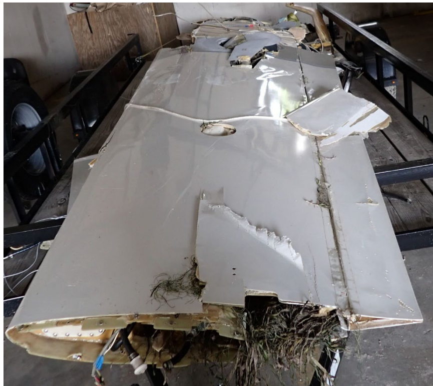
Figure 5 View of Nearly the Entire Span of the Wing and Carry-Thru Structure
